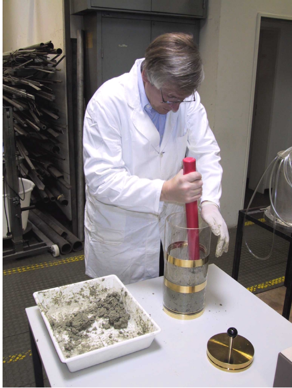
Figure 6-4: Placement of moisturized backfill into measurement cell for determination of material resistivity
