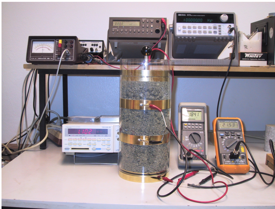
Figure 6-5: Measurement set-up for determination of backfill resistivity
