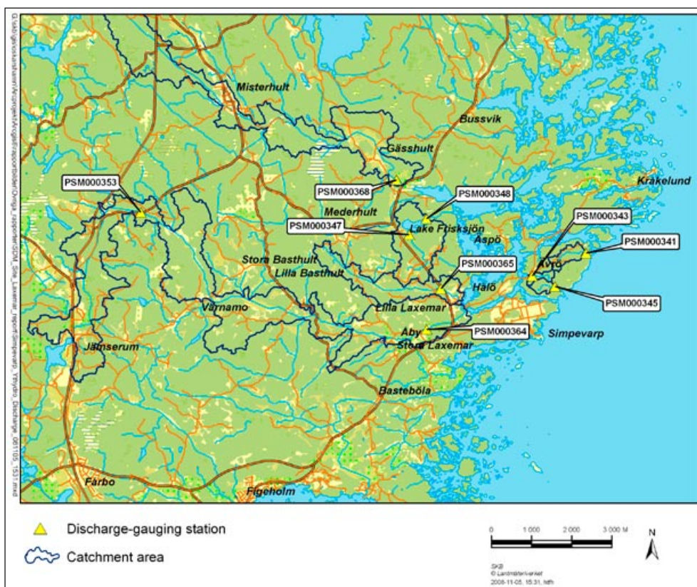
Figure 2-5. Overview map of discharge-gauging stations and their associated catchment areas, as determined from the DEM.
