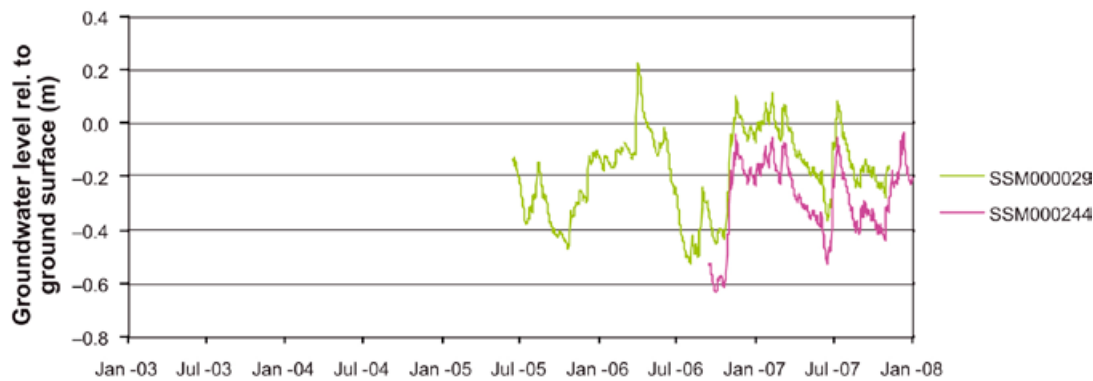
Figure 3-29. Time-series plot of daily average groundwater levels below the Kärrsvik wetland.
