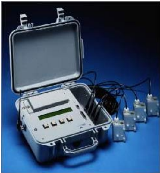
Figure 3-2. Recording unit Ava95 and geophones for vibration measurement.
