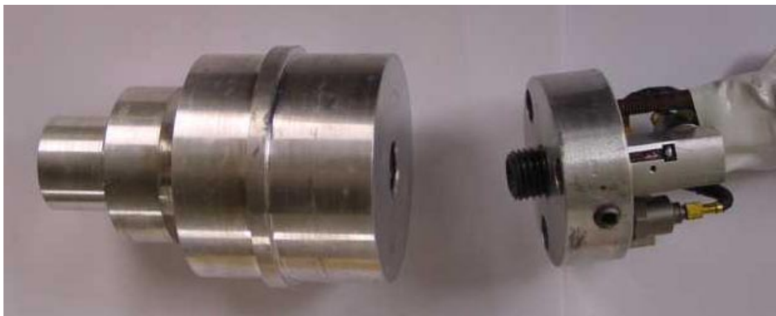
Figure 3-8. Photo of accelerometers, base plate and anchor (from right to left).
