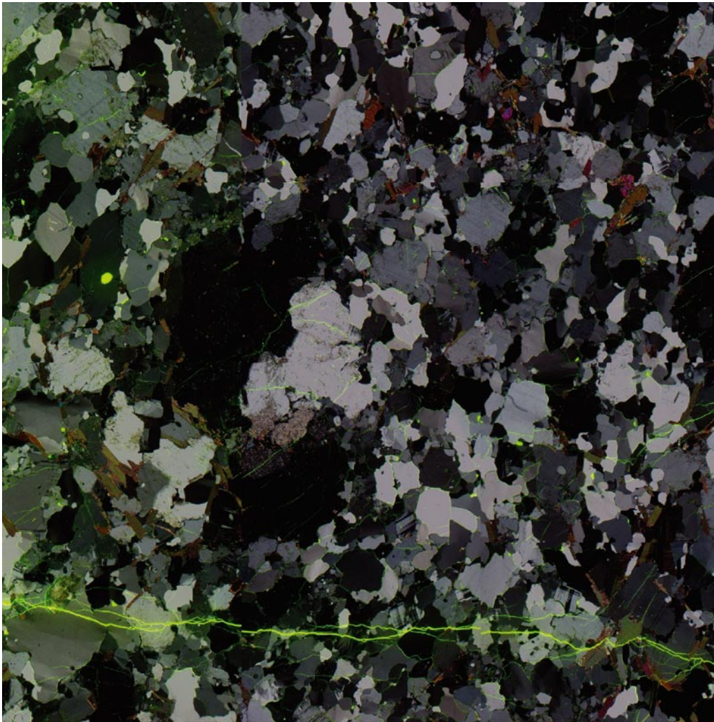
Figure 4-14. Combined polarised and fluorescent microscopic image of specimen F4B2. Image size is 8.3 x 8.3 mm.
