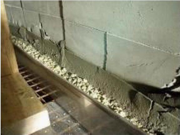
Figure A-8. Wetting of the granules and base of blocks (144 hours) (note lower layer of wet blocks and their deformation due to mass of overlying material).
