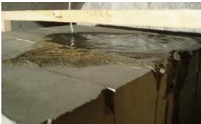
Figure A-5. Water and eroded clay flowing down the side of Test 2 (note also the swelling of clay blocks on left side of photo cause water to flow to right).
