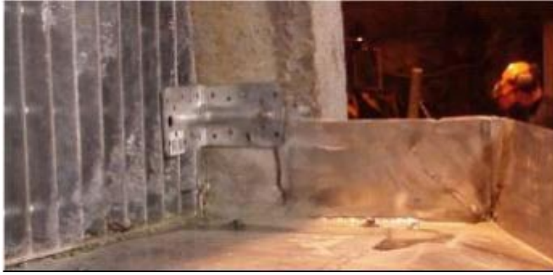
Figure A-48. Water exiting lower corner of Test 12 at 2.5 hours
