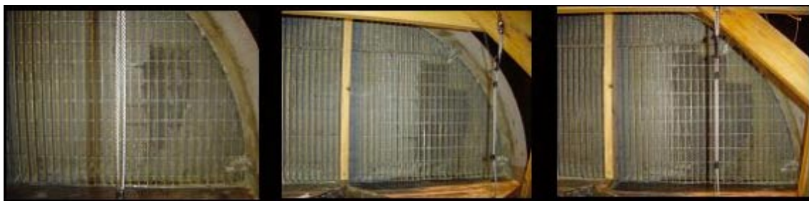
Figure A-65. Wetting patterns at face of Test 29 during testing.
