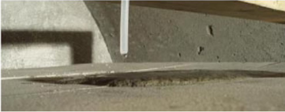
Figure A-4. Water supply to and rapid swelling of clay (note swelling of clay and pooling of water above it).
