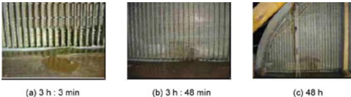
Figure A-58. Wetting at face of Test 27.
