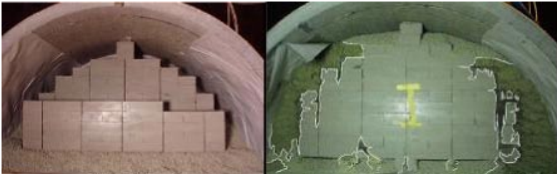
Figure 7-13. Closure of vertical construction gaps in Tests 9, 10.
