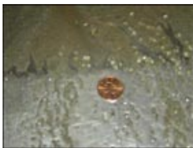
Figure A-60. Coarse particulate materials eroded from Test 27. (Note coarse, weakly cemented white particles and finer dark eroded materials).
