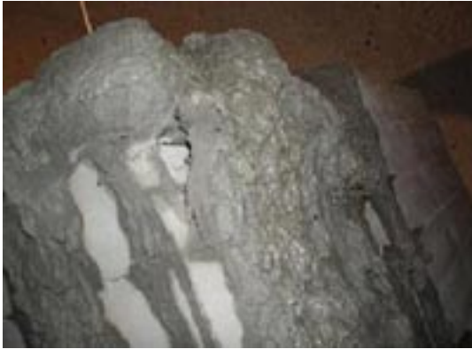
Figure A-6. Erosion of block assembly (24 hours after start) (extensive swelling of clay and slumping from top of assembly).
