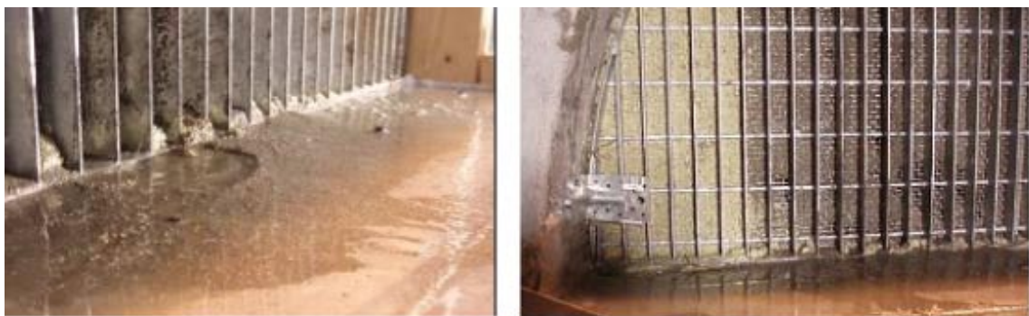
Figure A-18. Eroded materials and water outflow from Test 11.
