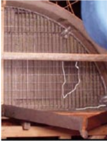
Figure A-43. Test 14 at 5 hours, showing where water outflow was observed.
