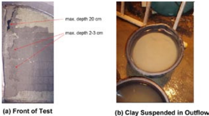
Figure A-50. Erosion of clay from Test 16.
