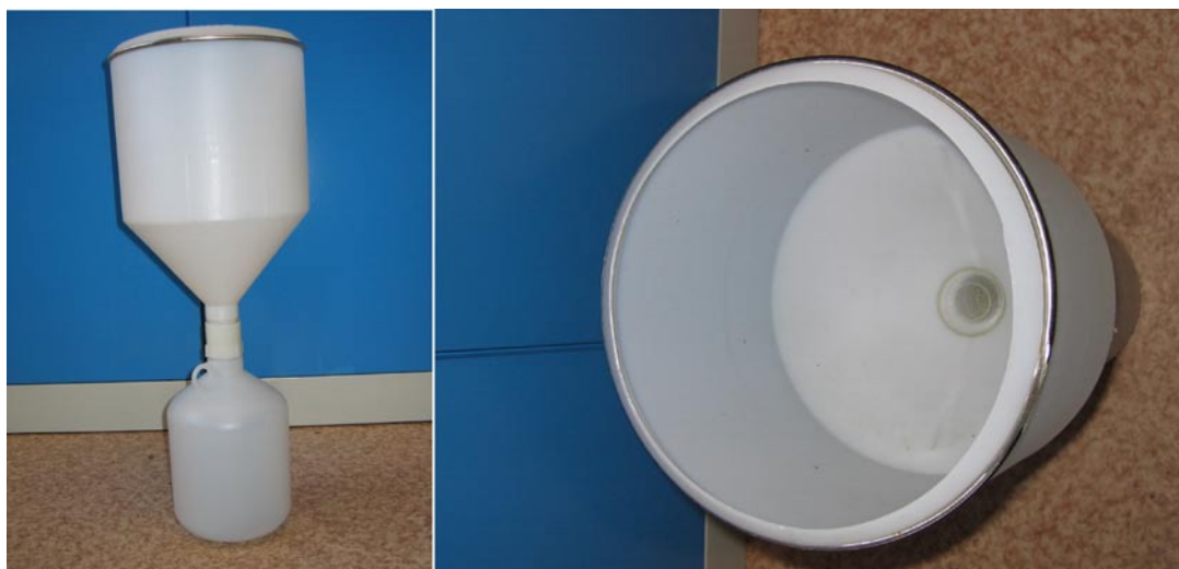
Figure 3-1. The sampler used in summer at the site for sampling of precipitation at the island of Åspö.
