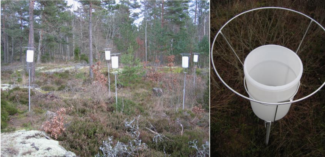
Figure 3-2. The sampler used in winter at the site for sampling of precipitation at the island of Äspö.
