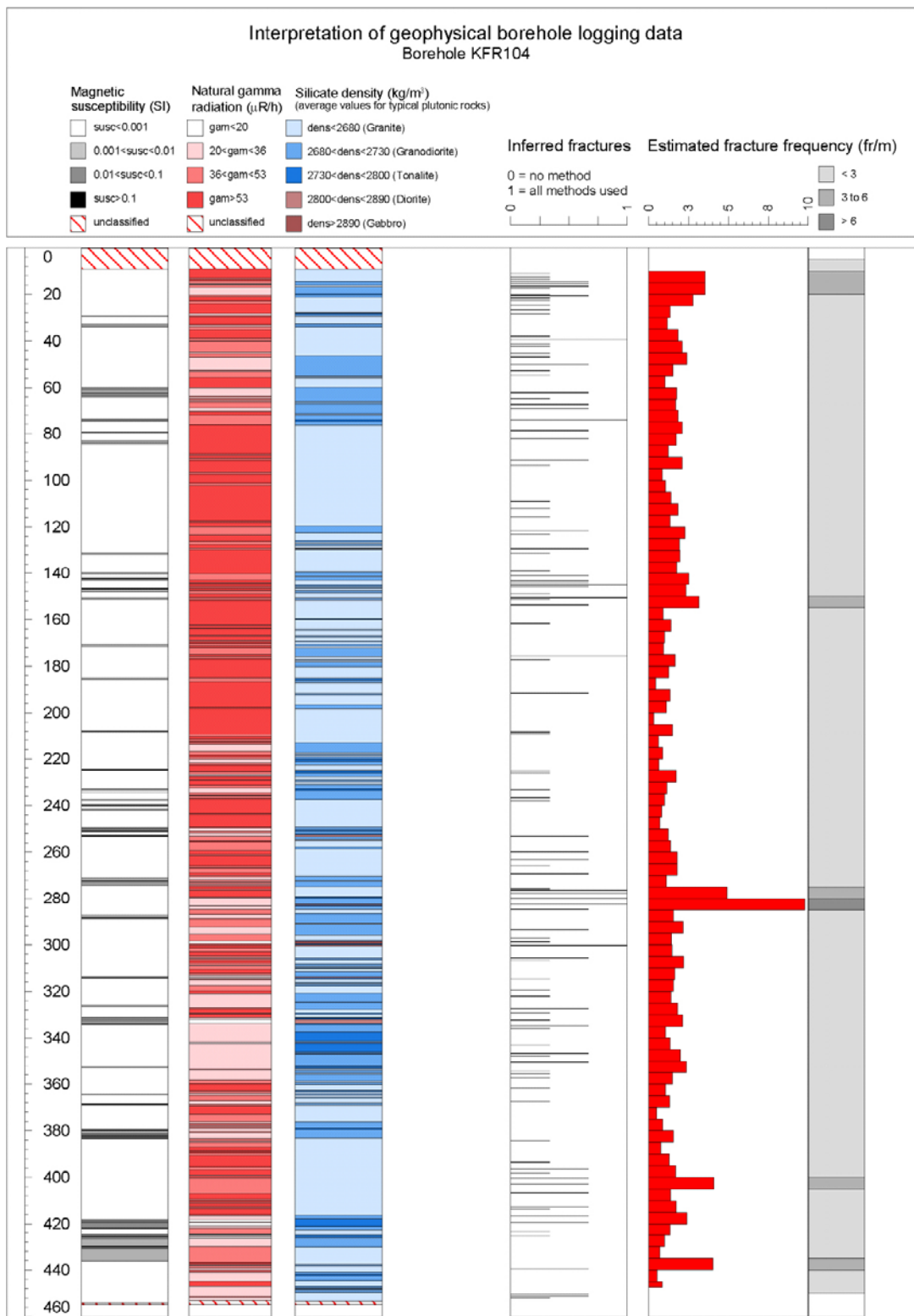
Figure 5-4. Generalized geophysical logs of KFR104.
