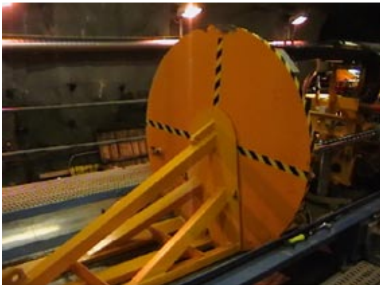
Figure 5-15. Distance frame for transportation of Distance Blocks.
