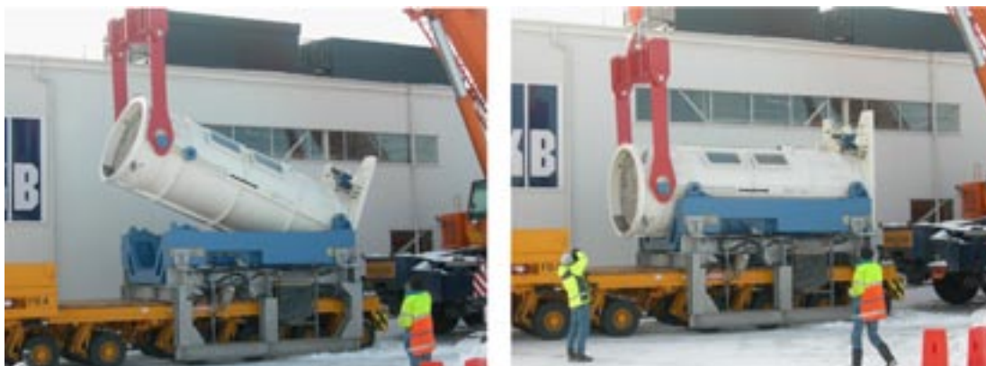
Figure 4-28. Tilting of the transport tube. Only the heavy gamma gate is mounted to the transport tube.
