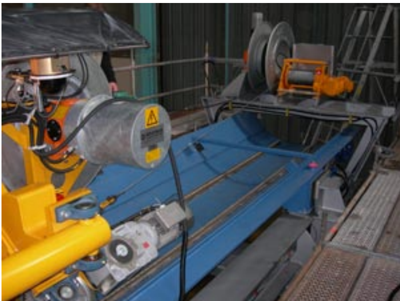
Figure 4-14. Winch for retraction of the machine.
