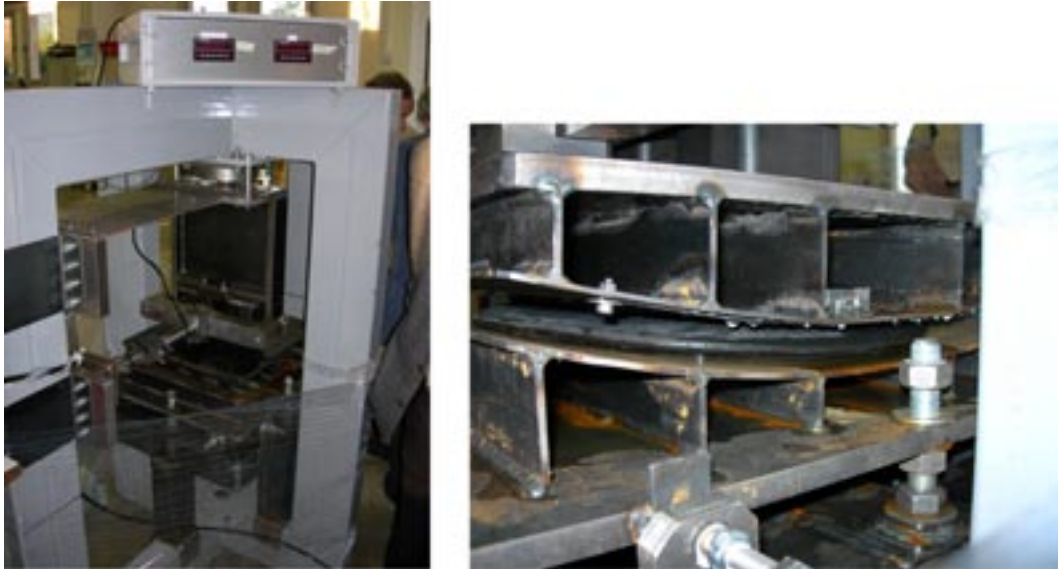
Figure 4-18. Test bench for cushions at ECA's premises.
