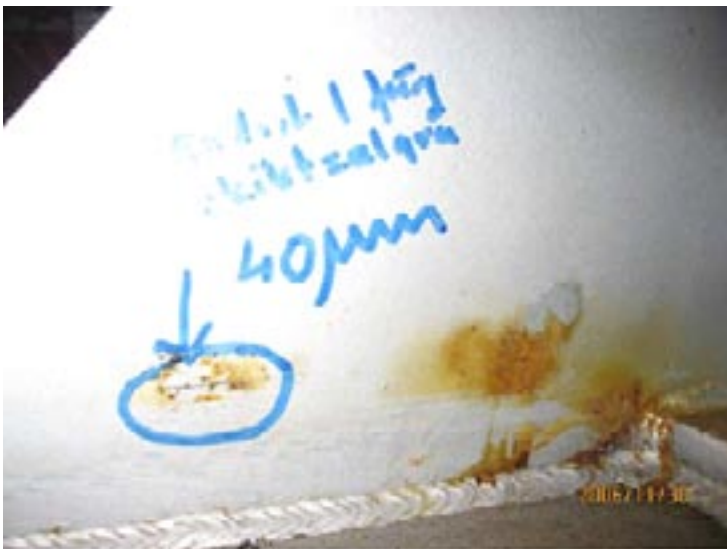
Figure 5-14. Example of the quality of the surface protection on the transport support for the deposition machine.
