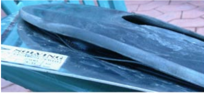
Figure 5-6. Broken cushion due to high pressures.
