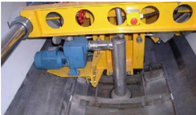
Figure 5-9. Water recovery pump and suction nozzle.
