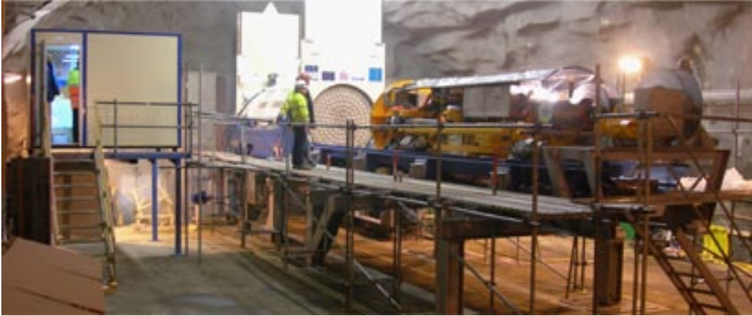
Figure 5-2. Set-up of equipment at the test site at Äspö HRL, level -220 m. The Supercontainer is inside the transport tube with the shielding gamma gates open. The control room is on the left side on this photo.
