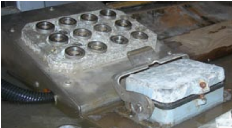
Figure 5-13. Connection block for water supply lines on the pallet.
