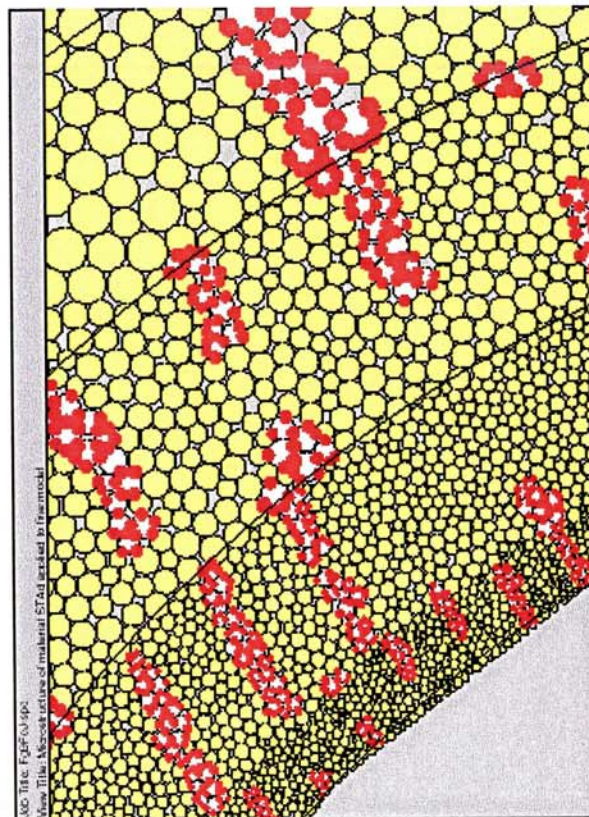
Figure 26. Discrete anisotropy material STAd applied to the fine-resolution test-hole model.
