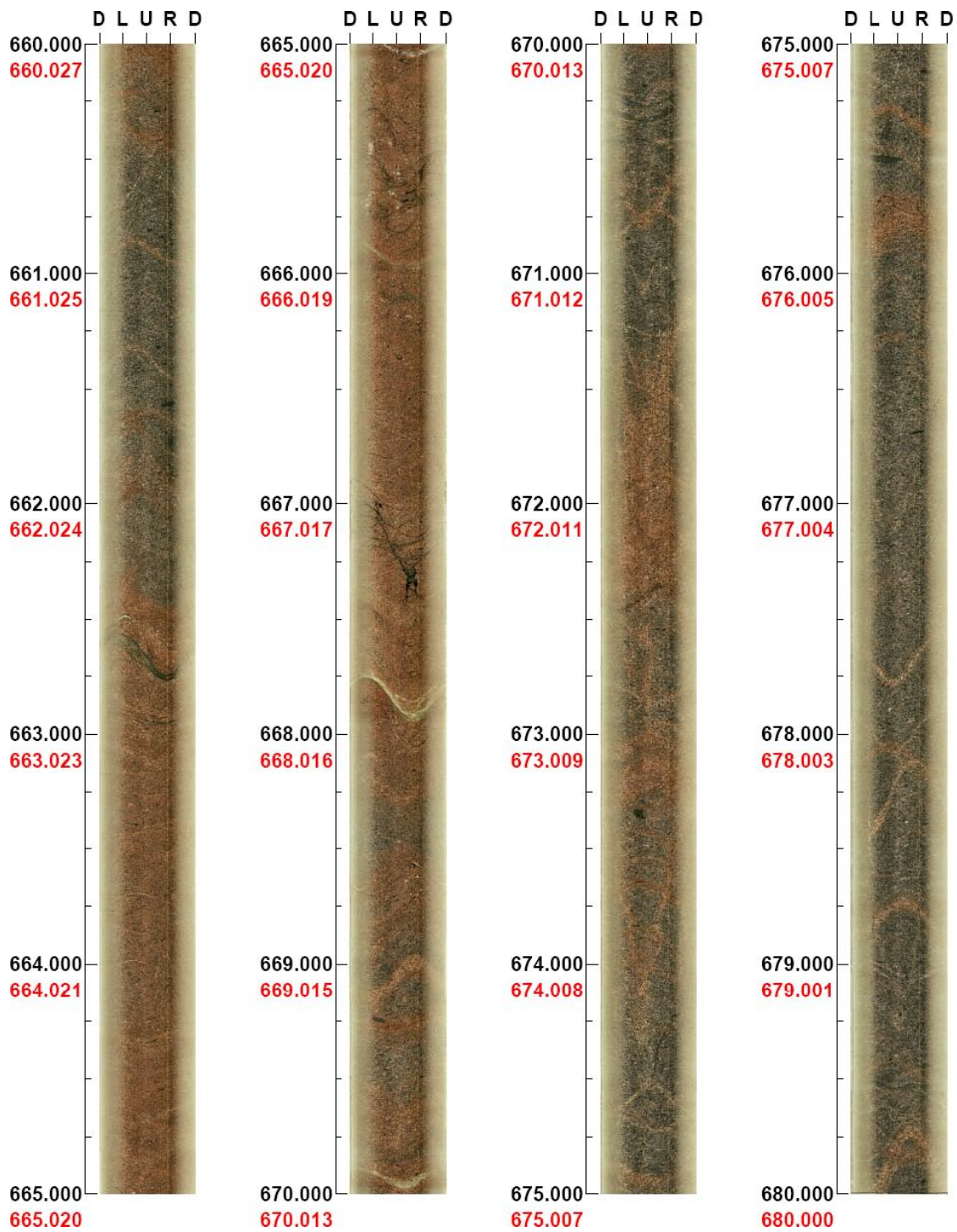
Figure A3-2b. Borehole KLX17A: selected BIPS logging image from 660 to 680 m including the water bearing fractures at 642–701 m. The non-adjusted length is marked with black and the adjusted true length is marked with red /4/.
