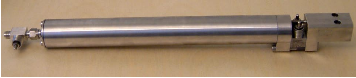
Figure A8-3. SKB stainless steel sampling cylinder (left: piston side, right: mounting adapter side).
