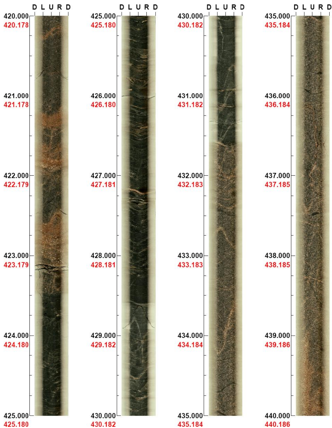
Figure A3-1b. Borehole KLX17A: selected BIPS logging image from 420.0 to 440.0 m including the water bearing fractures at 416–437 m. The non-adjusted length is marked with black and the adjusted true length is marked with red /4/.
