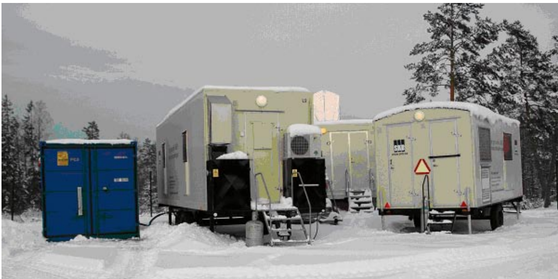
Figure 4-1. The mobile units used at KLX17A; from left container for collecting the water from the borehole, laboratory unit, hose unit with downhole equipment and a unit for computer work.
