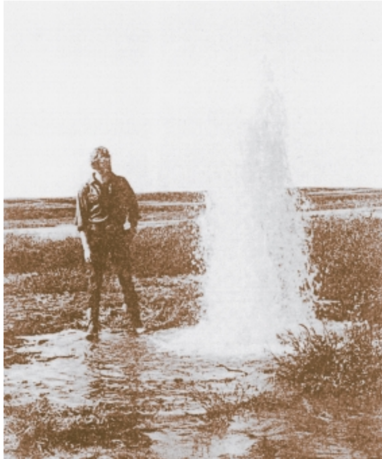
Figure 3-2. Photograph of artesian flow from borehole drilled into side of pingo /from Mackay, 1978/.
