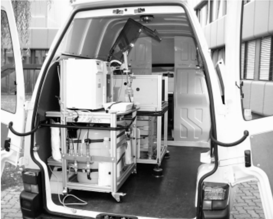
Figure 3-5 The equipment for Laser-induced Breakdown-Detection (LIBD) of colloids is installed in a van in order to allow mobility and on-line measurements in boreholes.
