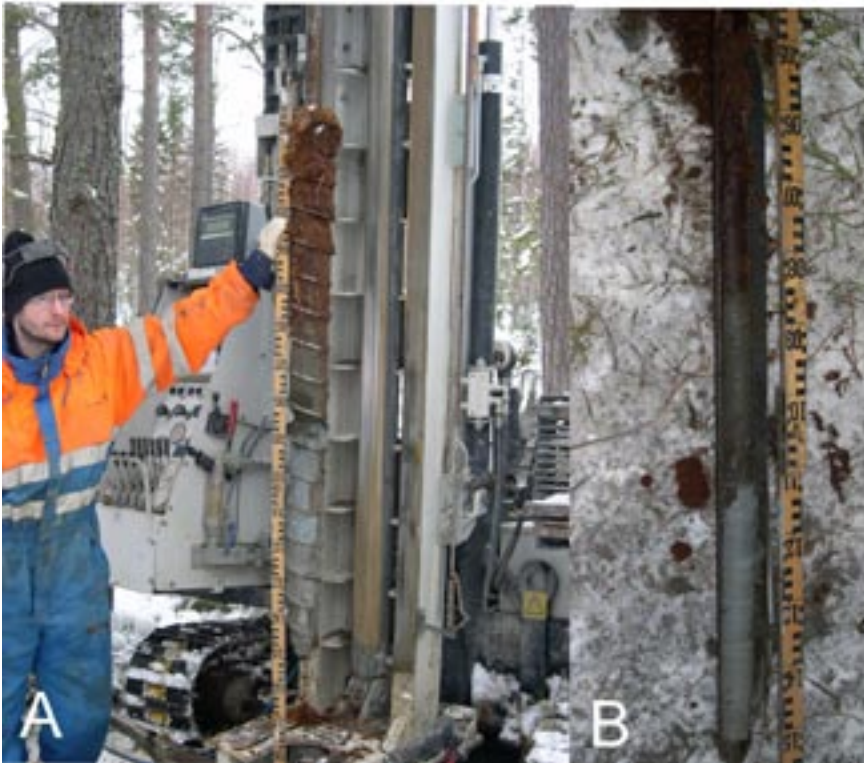
Figure 5-53a. The geotechnical drilling rig with a sample showing a part of core SFM0095 (c. 1–2.5 m depth). The lithostratigraphy is from the top: peat, reed peat, algal gyttja, clayey gyttja, sand, varved glacial clay. b. A sediment core collected using a Russian peat corer covering 1.5–2.5 m at SFM0095 /from Lokrantz and Hedenström 2006/.
