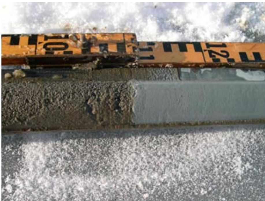
Figure 5-63. Part of the lithological sequence from the sampling site at Lake Eckarfjärden. Down is to the right where clay was obtained. Note the erosive contact between the clay and the sand, representing a hiatus of approximately 9,000 years. The upper part of the core consists of gyttja and is not presented in this picture.
