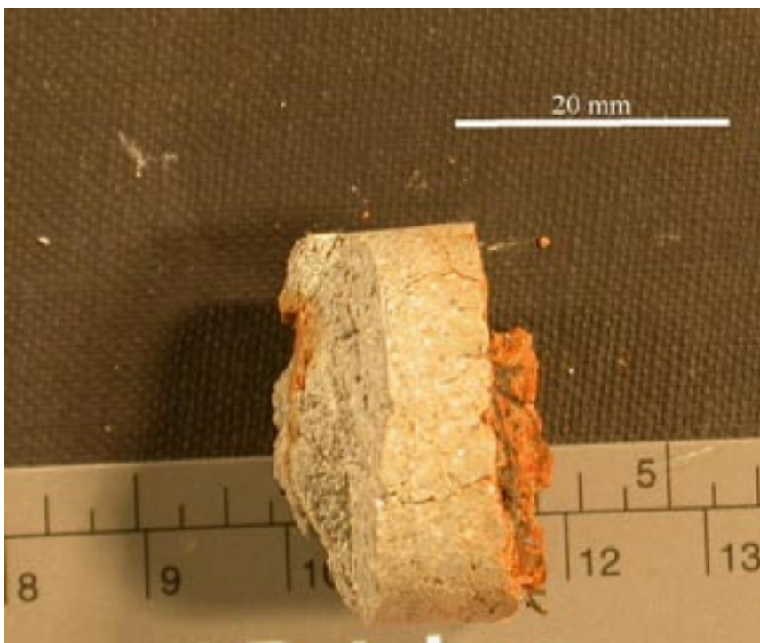
Figure 4-13. Photograph of subsample 16a showing interface between bentonite and 'bentonite with steel wire' region (right), and interface between bentonite and iron coupon (left). Reddish brown staining permeates the matrix of the bentonite between the steel wires but there is only very limited penetration of 'iron staining' into the adjacent the wire-free bentonite. Experiment NFC16.
