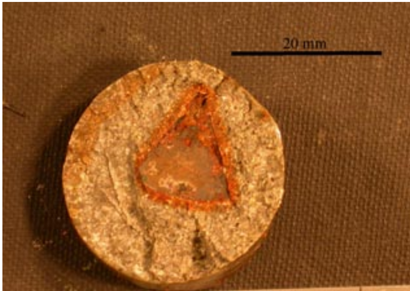
Figure 4-4. Photograph of subsample 12a sliced through the contact of the iron coupon near the unaltered end of the compacted bentonite cylinder (iron coupon removed), showing the 'triangular' mouldic impression of the segment of iron coupon. The coupon surface is coated with a film of reddish-brown iron oxide corrosion product and surrounded by thin halo of reddish-brown iron oxide staining in the immediately adjacent bentonite. Localised weak staining by orange-brown alteration can be seen in the outer margins of the sliced bentonite disc. Experiment NFC12.
