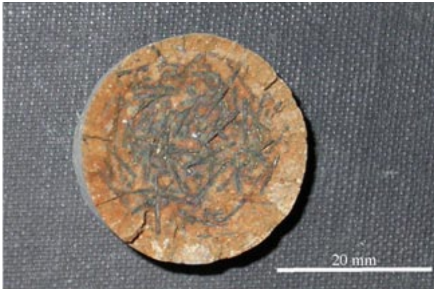
Figure 4-14. Photograph of subsample 16a showing the surface of the interface between bentonite and 'bentonite with steel wire' region. Reddish brown staining permeates the matrix of the bentonite between the steel wires but locally there are patches of iron-stain-free bentonite. The surfaces of the steel wires can be seen to be coated with a black oxide alteration product. Experiment NFC16.
