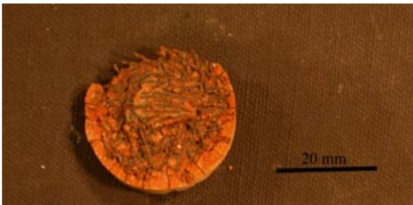
Figure 4-3. Photograph of subsample 12c sliced from the centre of the steel wire region of the compacted bentonite. The corroded wire surfaces are coated with a black iron oxide corrosion product, surrounded by narrow haloes of reddish-brown iron oxide alteration product. The adjacent bentonite matrix is strongly stained orange-brown. Note that shrinkage and cracking of the bentonite has occurred around the wire-free margin of the slice, whereas, the centre of the disc contaminating the wires displays markedly less shrinkage cracking. Experiment NFC12.
