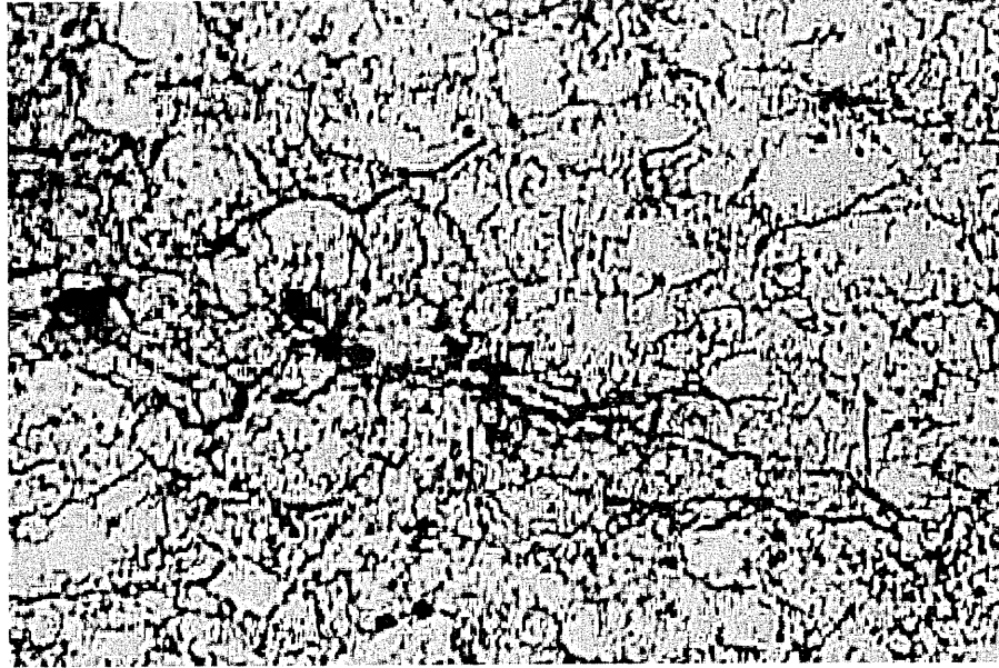
Figure 3.5-3. Audioradiogram of the section of rock sample B4 shown in Figure 3.2-1 as a thin section. The darker, fracture-like features are areas of increased porosity.
