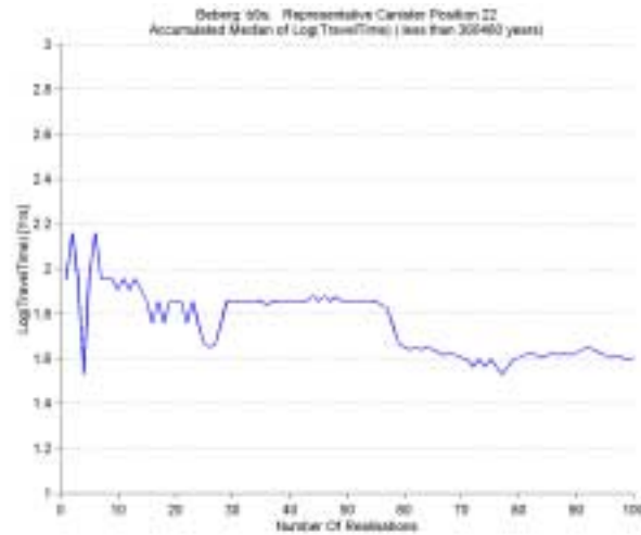
Figure 5-27 Monte Carlo stability at starting position 22. Cumulative median \log_{10} travel time versus number of realisations. Results for 100 realisations and a flow porosity of \varepsilon_f = 1 \cdot 10^{-4} .
