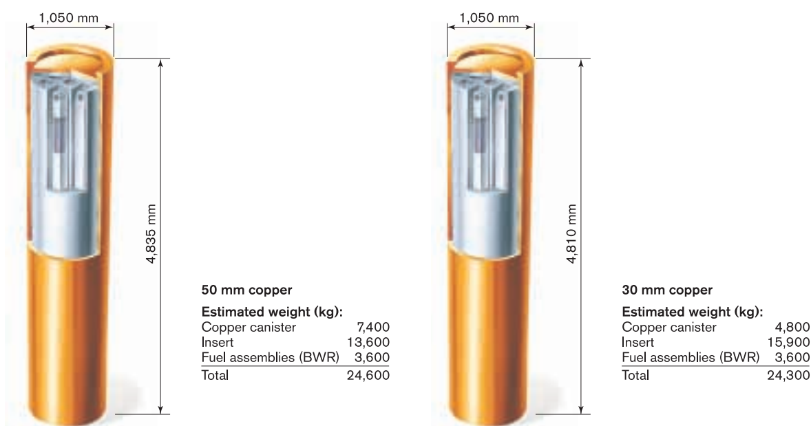
Figure 15-1. Dimensions and weights of canister with 50 mm and 30 mm wall thickness.
