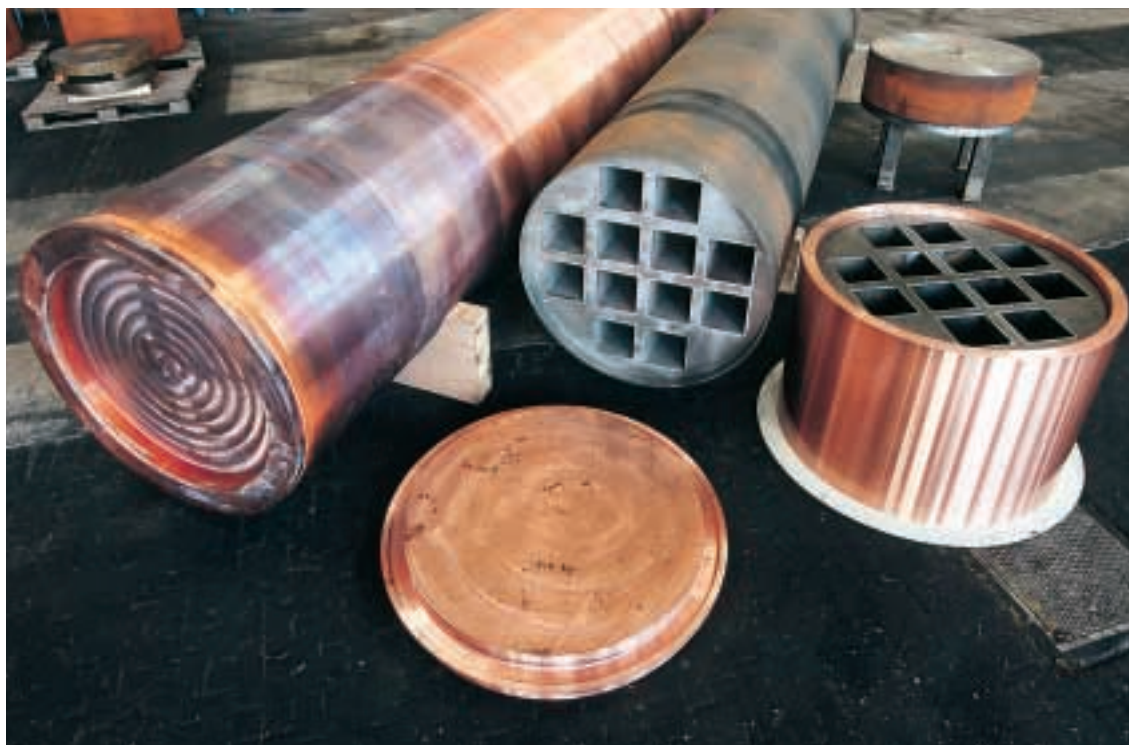
Figure 15-3. Examples of fabricated canister components and display objects.
