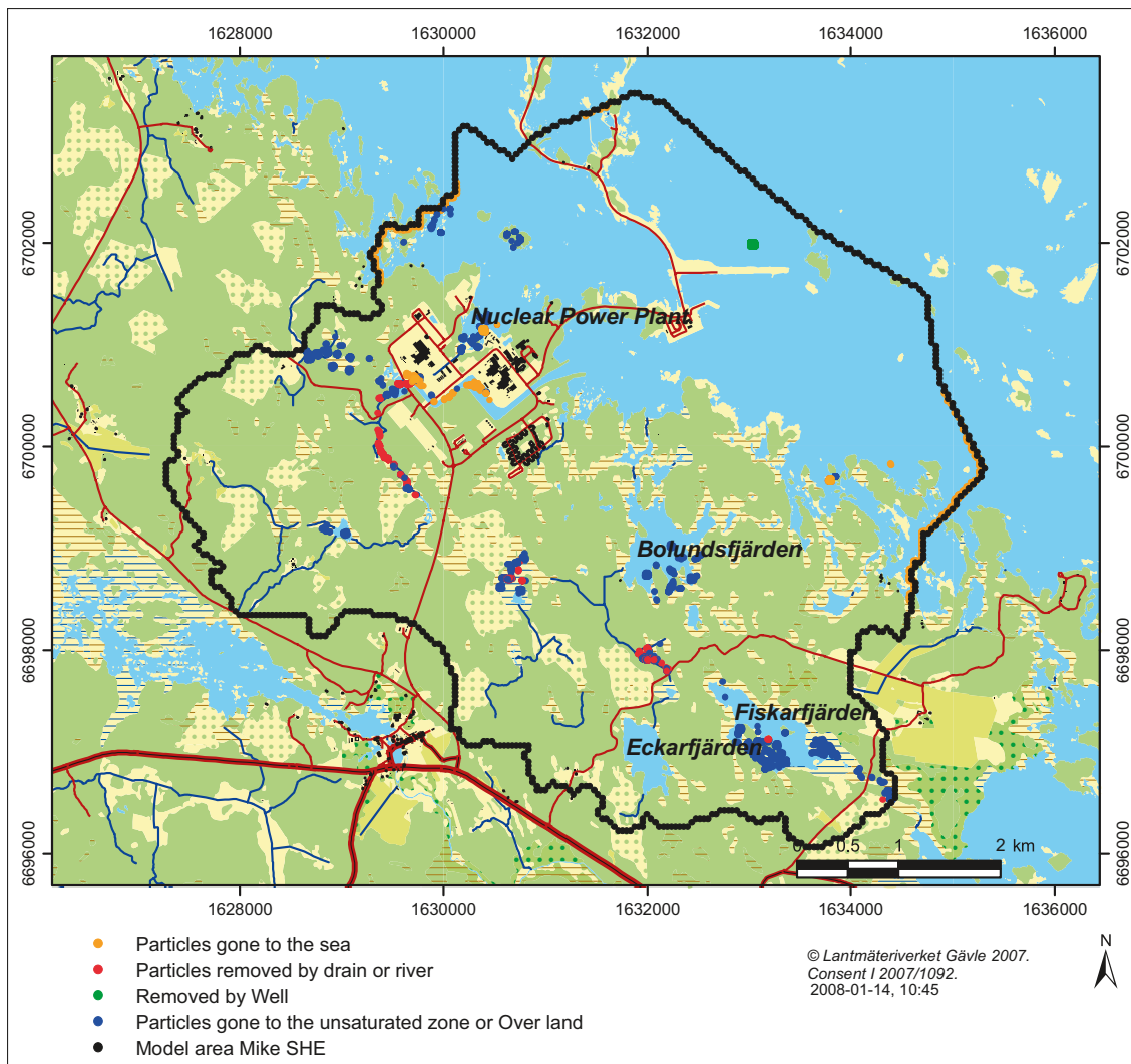
Figure 6-2. Sinks for the particles in case PT5-allover. The figure presents the results obtained with the SFR drainage activated in the model.
