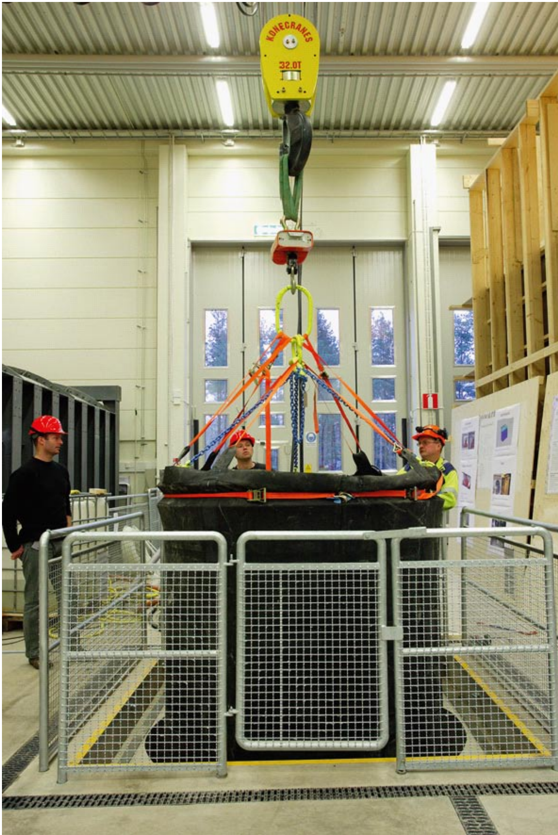
Figure 8-8. Detachment of the buffer protection sheet. It is being hoisted from the test hole in the picture.
