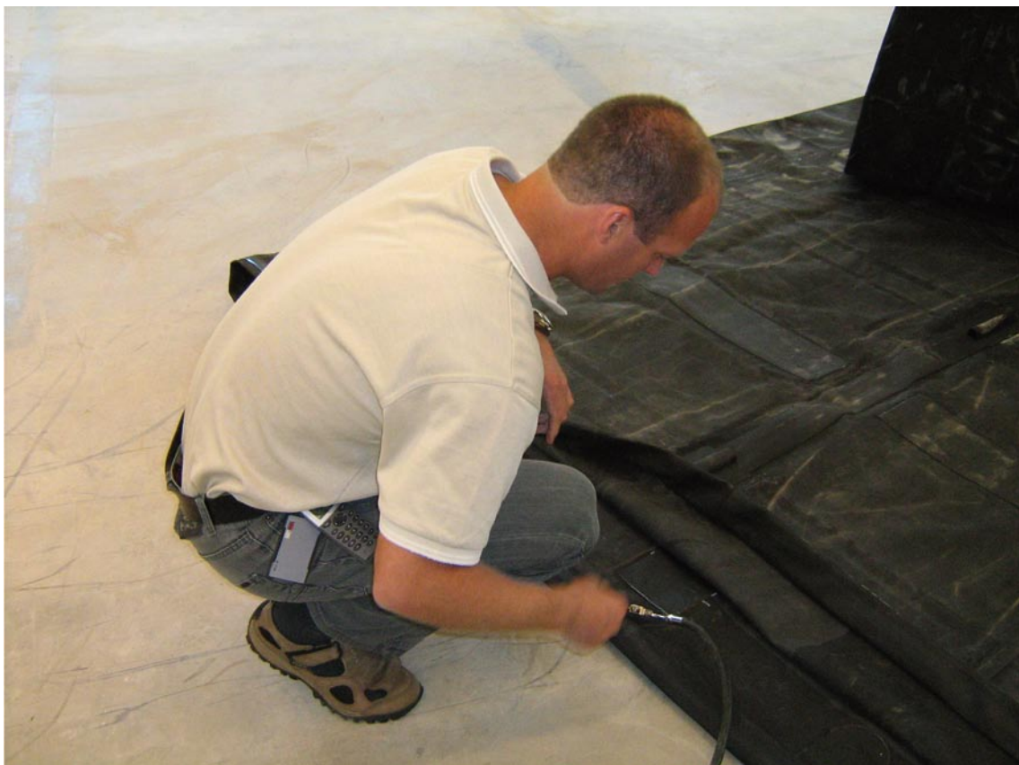
Figure 8-5. The buffer protection sheet with the tube for expanding it and the folded inflatable ring seal (held by the investigator).
