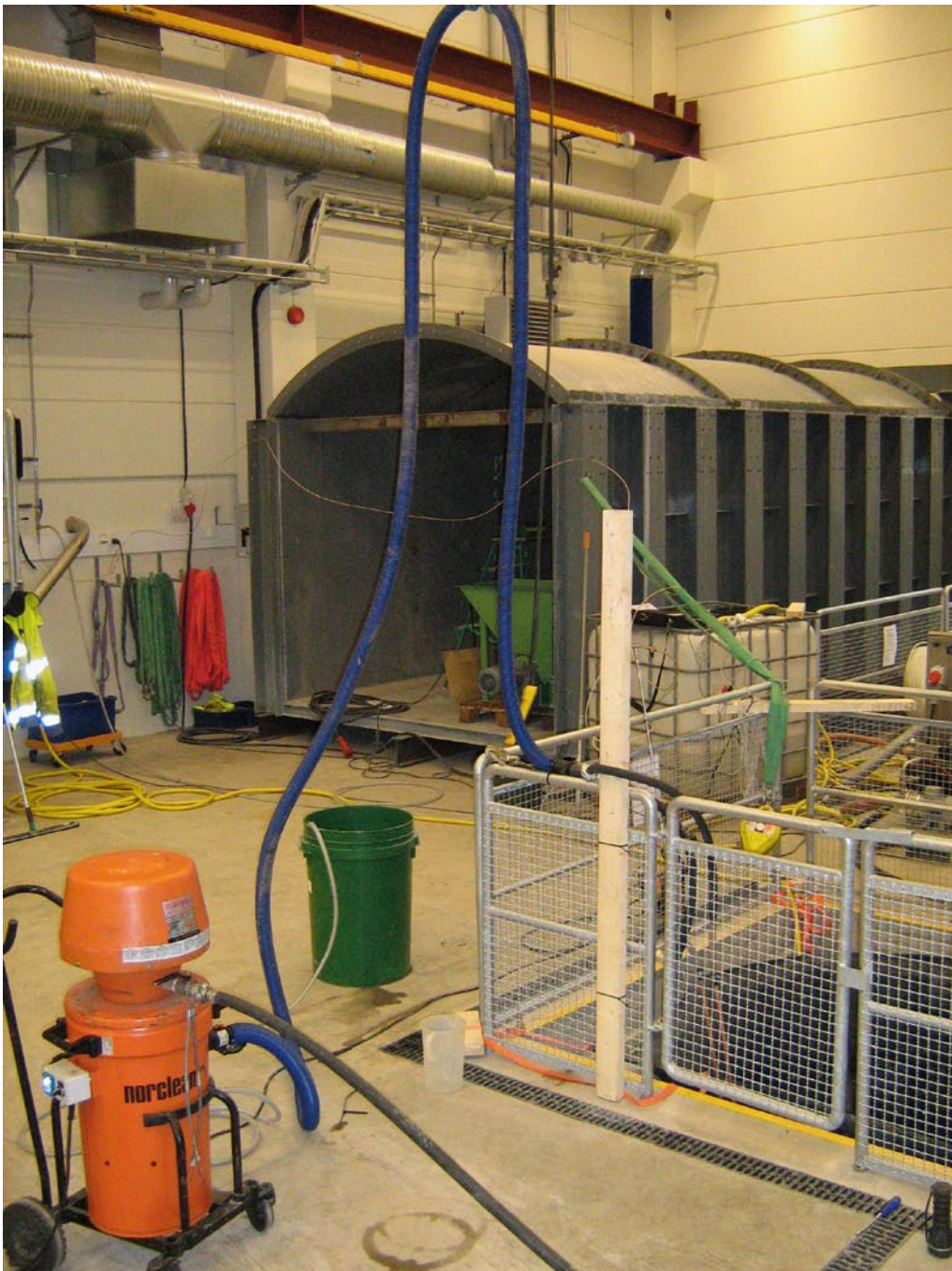
Figure 8-3. The vacuum pump (orange) with flexible tube (blue) connected to a tube (black) down to the bottom of the test hole.
