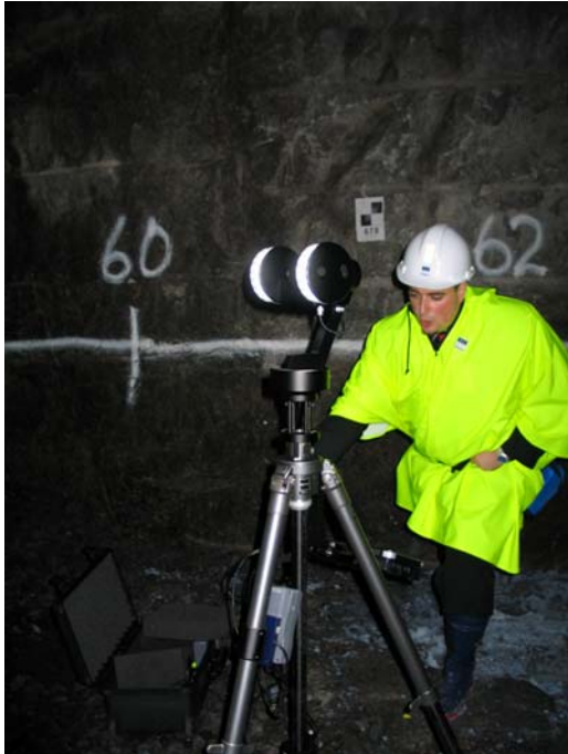
New equipment (SpheronCam HDR) is tested in the Tass-tunnel. (photo: Carljohan Hardenby)
