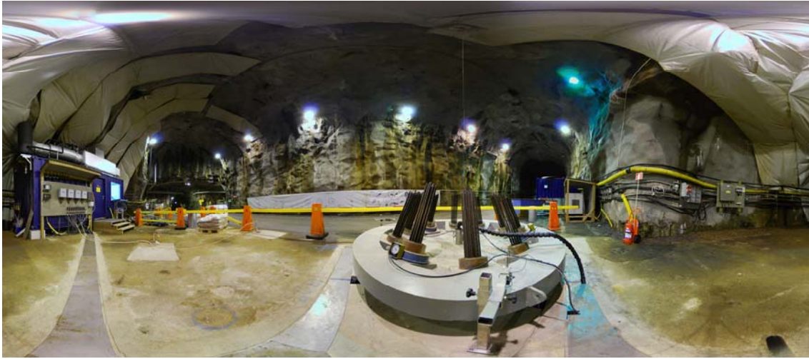
Panorama of the Large-scale gas injection test (Lasgit) 420 m below ground at Äspö HRL.
