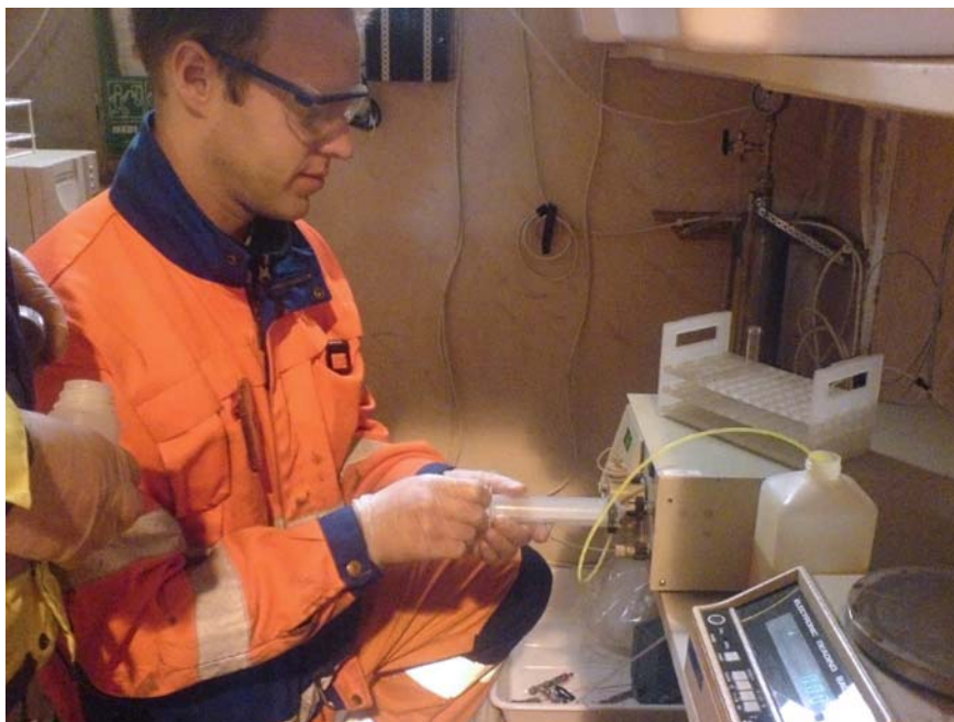
Injection of tracer in fracture
