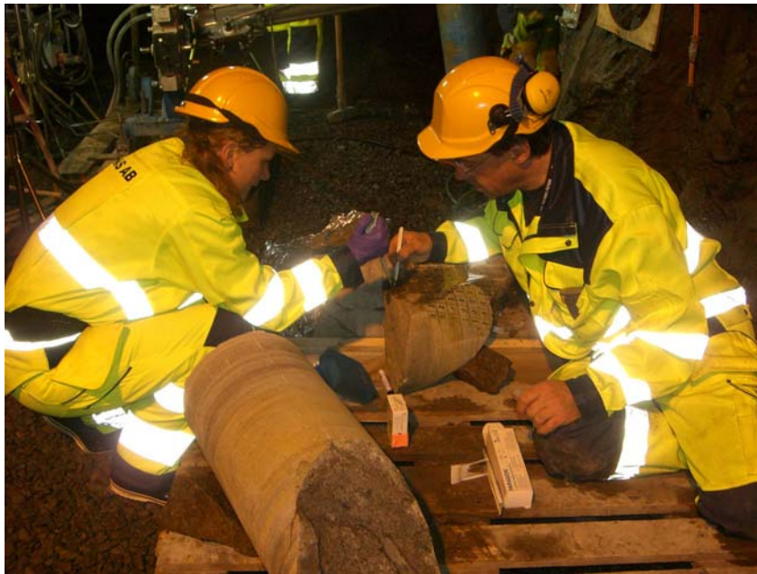
Sampling a new-drilled fracture surface for microbial presence and activity using DNA/RNA analysis methods.
