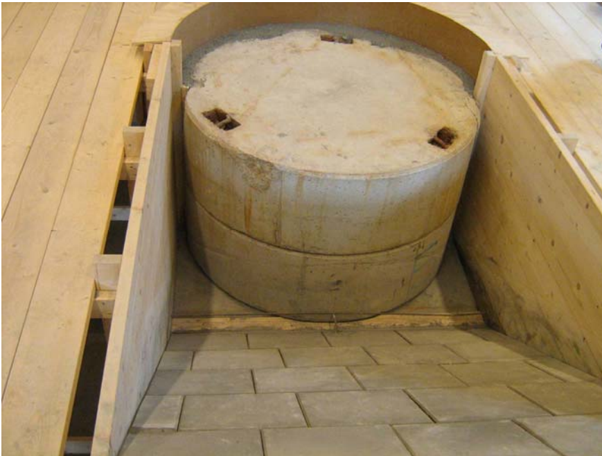
Figure 5-1. Test set-up for the bevel to the deposition hole.
