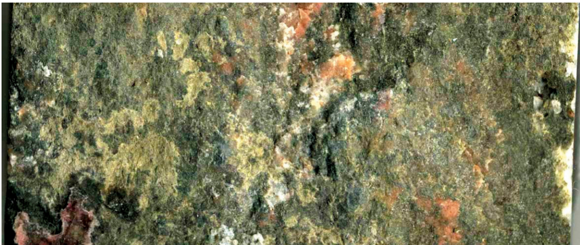
Figure 3-1. Fracture surface with thin coating of mainly chlorite, calcite, clay minerals and epidote. The length of the base of the photograph is 46 mm.
