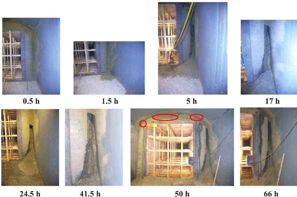
Figure A-21. Front face of Test 10 showing erosion of pellet materials.
