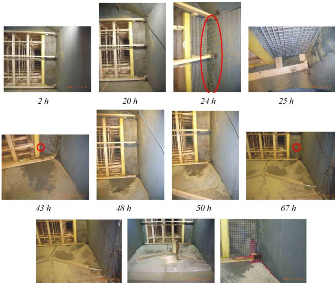
Figure A-27. Face of Test 12 at various times during water infiltration.
