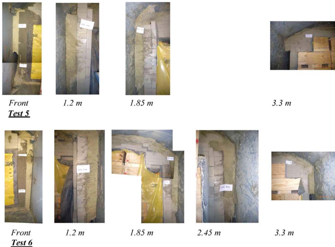
Figure A-10. Excavation profiles for Test 5 and Test 6. (note: incomplete wetting of pellets and movement of water into upper rear part of tests).
