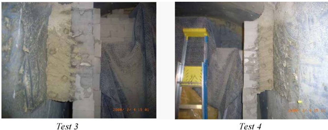
Figure 6-4. Wetting near Inflow location in Tests 3 and 4. (Note very limited extent of wetting and dark areas where limited water movement inwards along block joints occurred).
