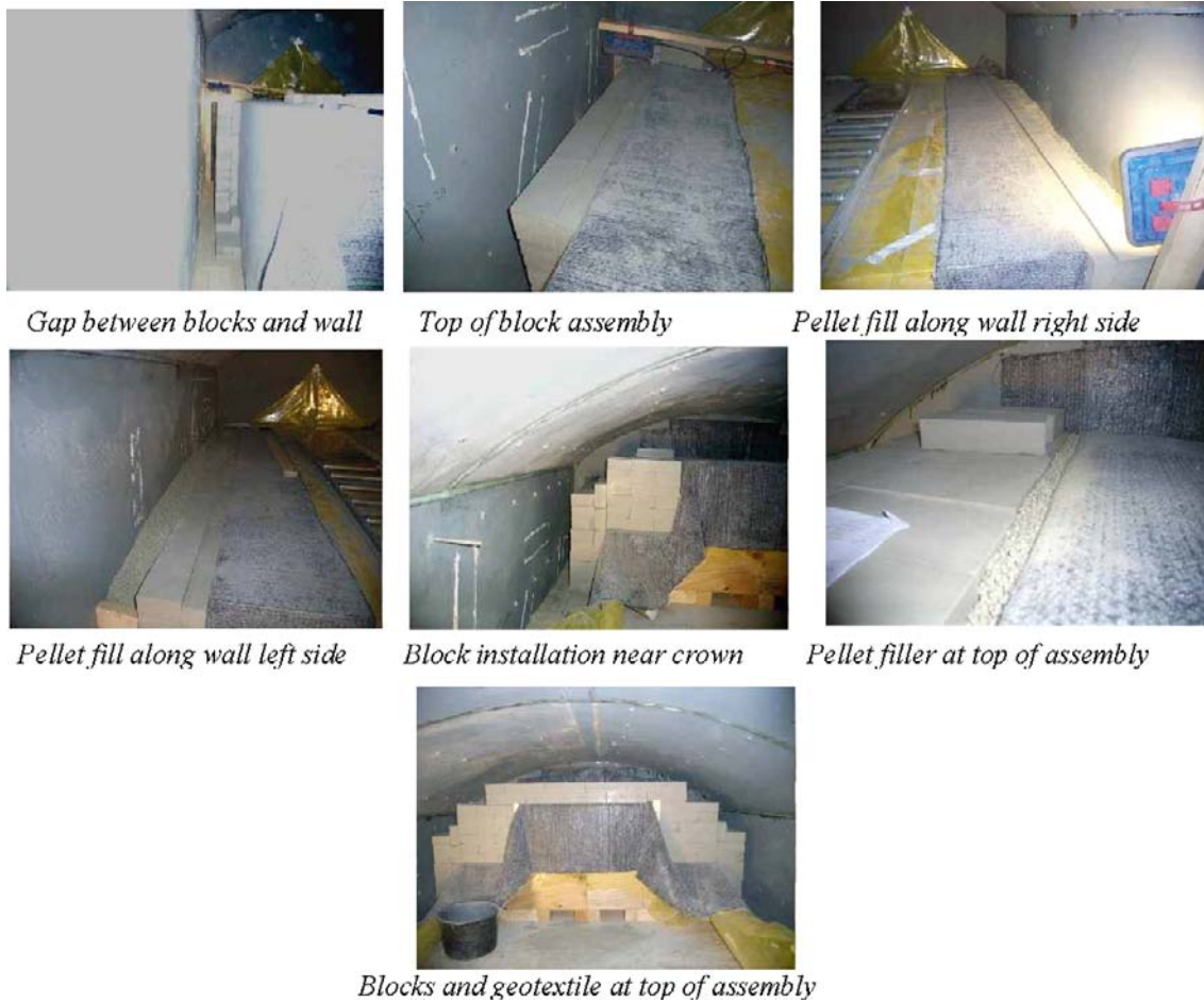
Figure 4-10. Construction steps for Assembly 1 (Tests 1, 2).
