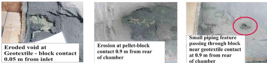
Figure 6-23b. Piping features initially present along pellet-block interface in Test 12.
