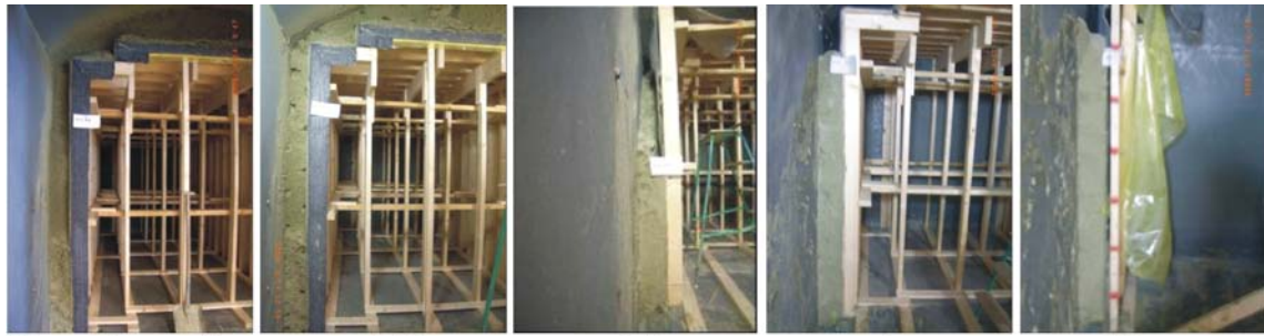
Downstream face ~0.15 m ~0.5 m ~1 m ~1.5 m (a) Wetting patterns observed at various distances from front face of Test 7
