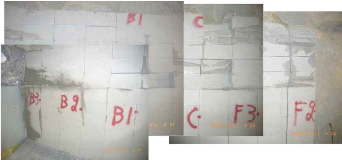
Figure A-5. Movement of water along block joints near top of Test 2. (Photomosaic view from rear (left) to front (right) along the block-geotextile boundary).
