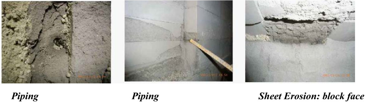
Figure 6-23a. Short-term erosional features observed in block-filled regions.
