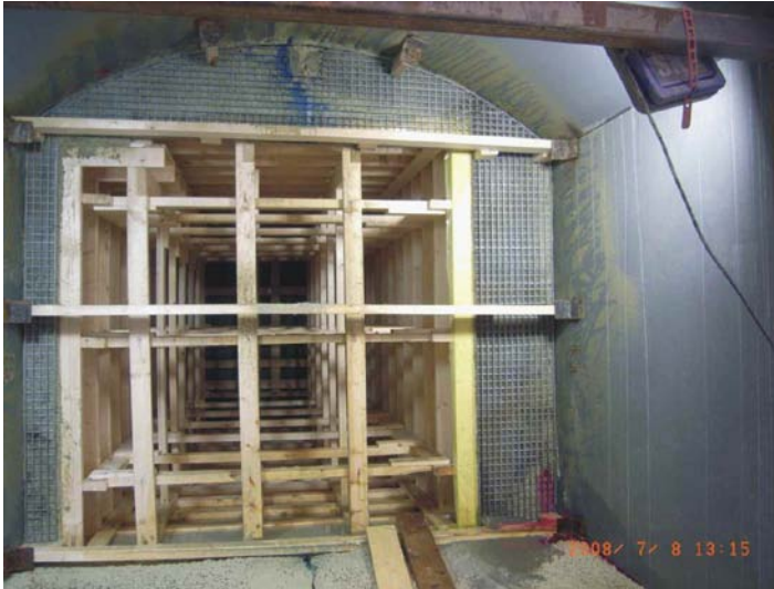
Figure 6-14. Assembly 6 (Tests 11 and 12) at the end of testing Test 12. (Note blue tracer exiting a crown of chamber).
