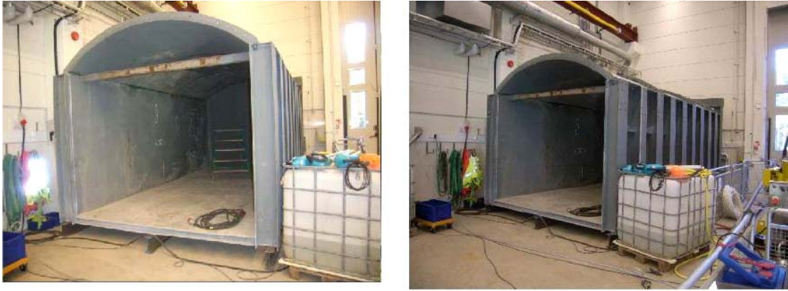
Figure 4-2. As-built 1/2-Scale test chamber.
