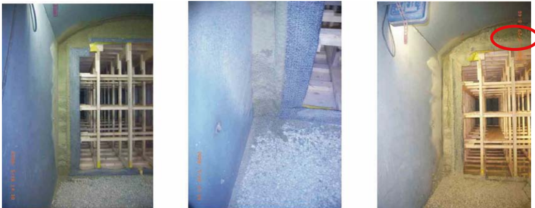
(a) Test 9 at beginning of water inflow and at time of dismantling (note water standing on floor of wooden framed volume)
