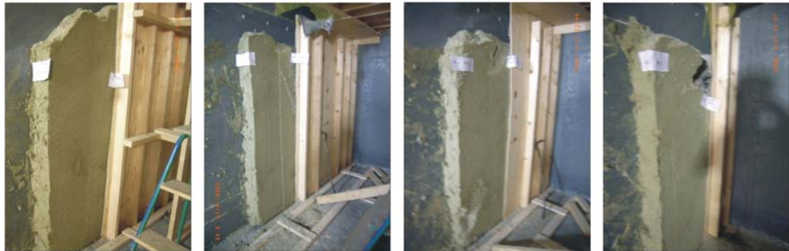
~0.5 – 1.5 m ~1.5 – 2.5 m ~2.5 – 3.5 m ~3.5 – 4 m (b) Wetting of pellet fill along walls of chamber following removal of dry pellets
