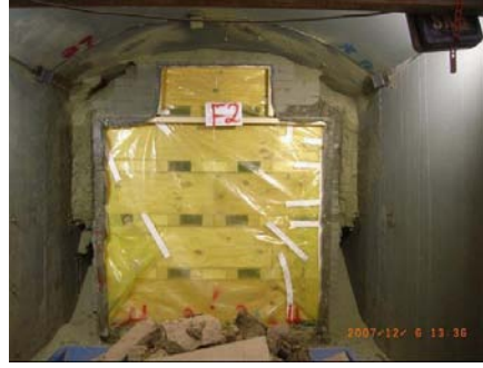
(b) Dry material at crown and base of assembly, just in from front face
