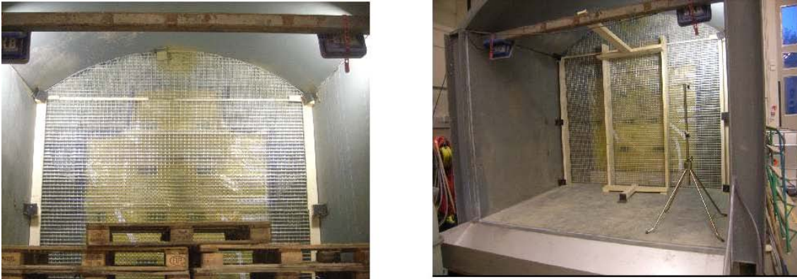
Figure 4-6. Mesh and Restraint at Downstream Face in Tests 1 Through 6.
