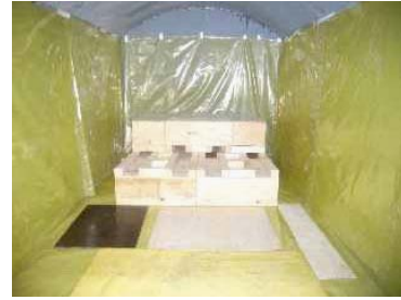
(c) Plastic liner & filler blocks
