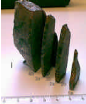
Figure 3-20. Wall rock sample structure #22 in KI0025F02:66.7m sawn parallel to fracture surfaces for autoradiography to provide porosity histograms at different depths.
