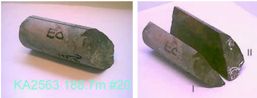
Figure 3-51. Wall rock sample structure #20 in KA2563:188.7m sawn perpendicular to fracture surface for autoradiography to provide profile measurements.
