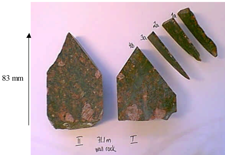
Figure 3-40. Sawings parallel to fracture surface of sample structure #21 in KI0023F:71.1m for autoradiography to provide porosity histograms at different depths. Length of sample is 83 mm.
