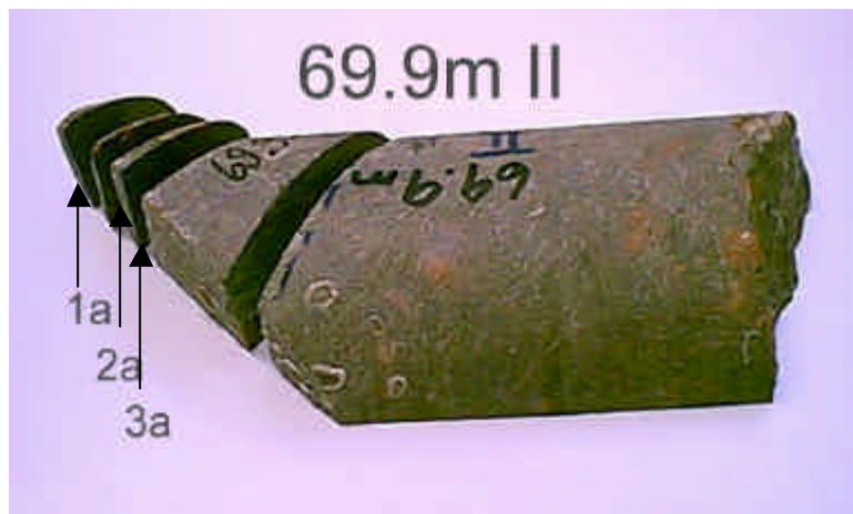
Figure 3-36. Sawings of wall rock sample II structure #20 in KI0023B:69.9m parallel to fracture surface for autoradiography to provide porosity histograms at different depths from fracture surface.
