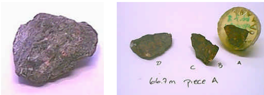
Figure 3-11. Sawings of piece sample A from structure #22 in KI0025F02:66.7m for autoradiography to provide porosity measurements.
