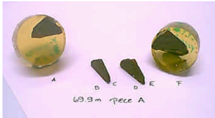
Figure 3-15. Sawings of piece sample A from structure #20 in KI0023B:69.9m for autoradiography to provide porosity measurements.
