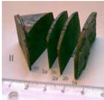
Figure 3-20. Wall rock sample structure #22 in KI0025F02:66.7m sawn parallel to fracture surfaces for autoradiography to provide porosity histograms at different depths.
