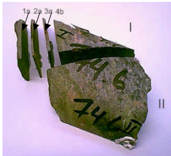
Figure 3-46. Wall rock sample #20 KI0025F02:74.6m sawn parallel to fracture surface for autoradiography to provide porosity histograms at different depths.
