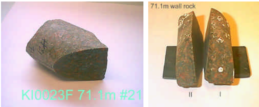
Figure 3-39. Sawings perpendicular to fracture surface of wall rock sample structure #21 in KI0023F:71.1m for autoradiography to provide profile measurements.
