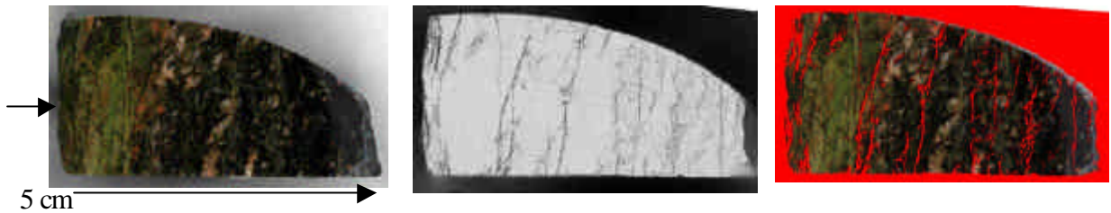
Figure 3-47. Photograph of wall rock sample II structure #20 in KI0025F02:74.6m (left), corresponding autoradiograph (center) (14 d exposure) and superimposed image (right) showing porous areas, where MMA has intruded. An arrow shows the fracture surface.
