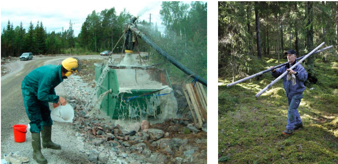
Figure 10-1. Two key features of the bedrock in the target area at Forsmark. Left: High water yields are often observed in the uppermost c 150 m of the bedrock. Right: The large number of unbroken drill cores gathered at depth support the observation of few flowing test sections in the deeper bedrock. (Figure 3-24 and Figure 3-34 in /Follin et al. 2007c/.)
