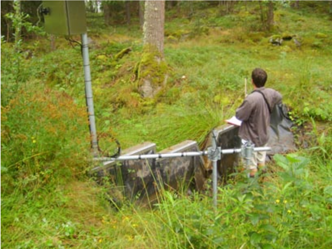
Figure 2-41. V-notch weir at gauging station PSM000345.
