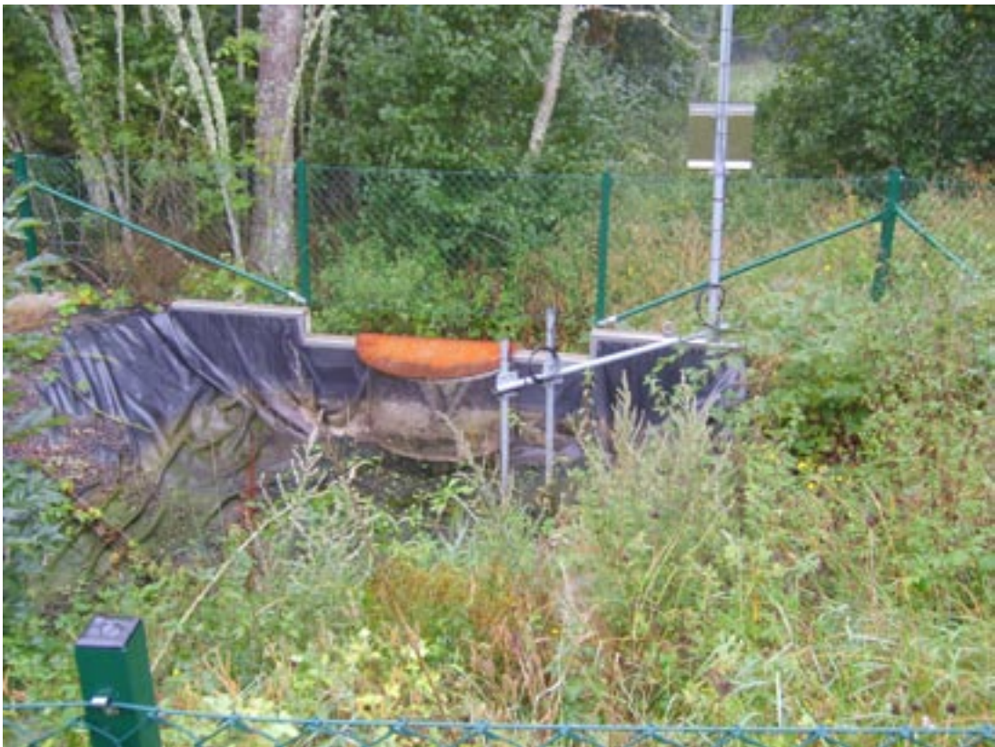
Figure 2-40. V-notch weir at gauging station PSM000343.
