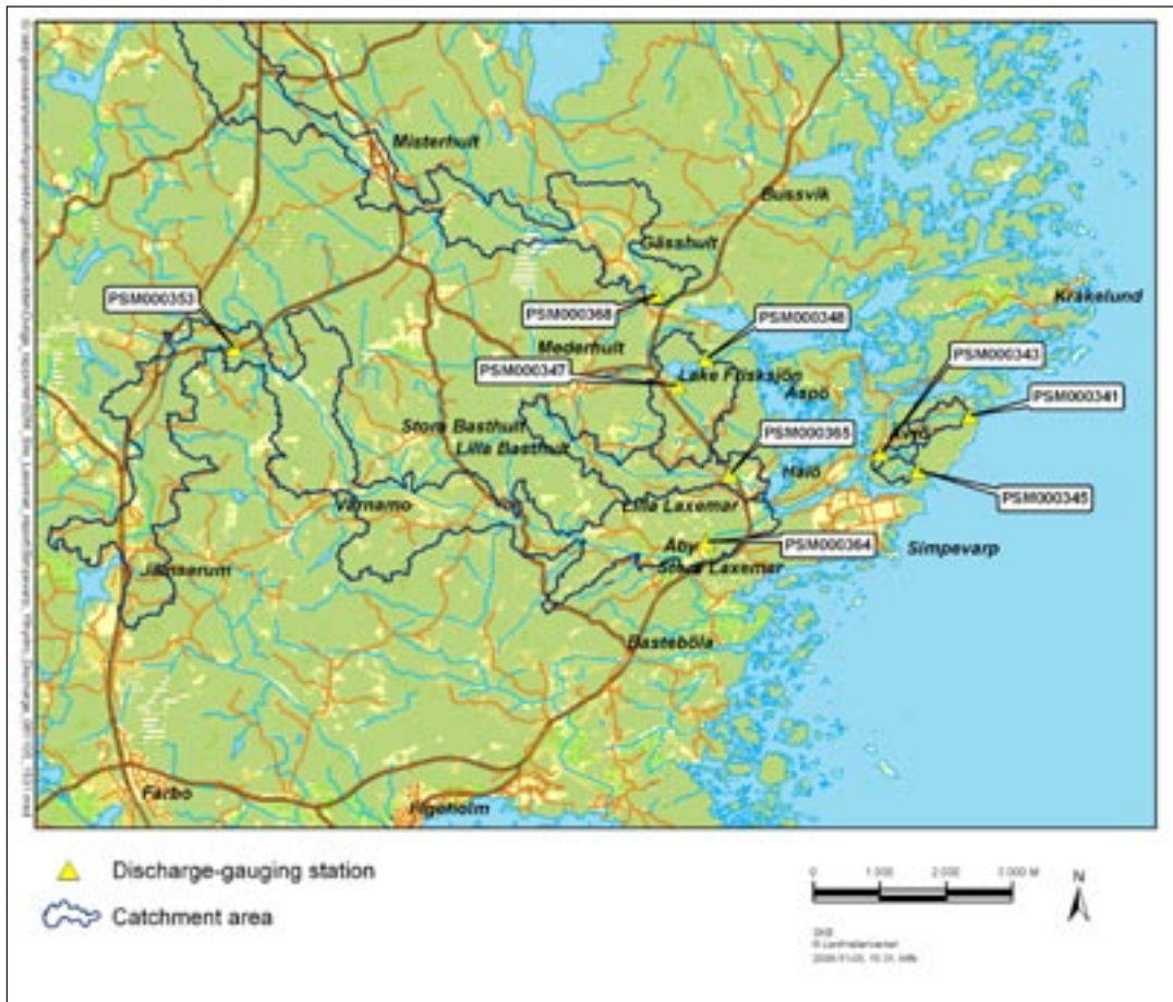
Figure 2-36. Overview map of discharge-gauging stations and their associated catchment areas, as determined from the DEM.
