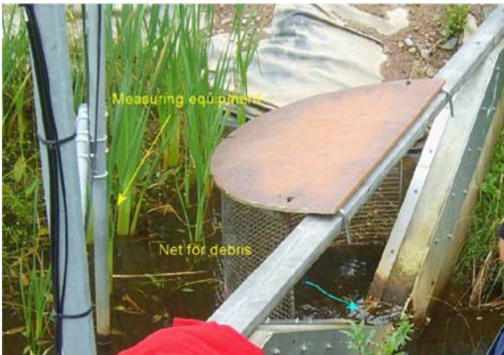
Figure 2-37. Design of the V-notch gauging stations (station PSM000365 in Ekerumsån is shown in the picture).
