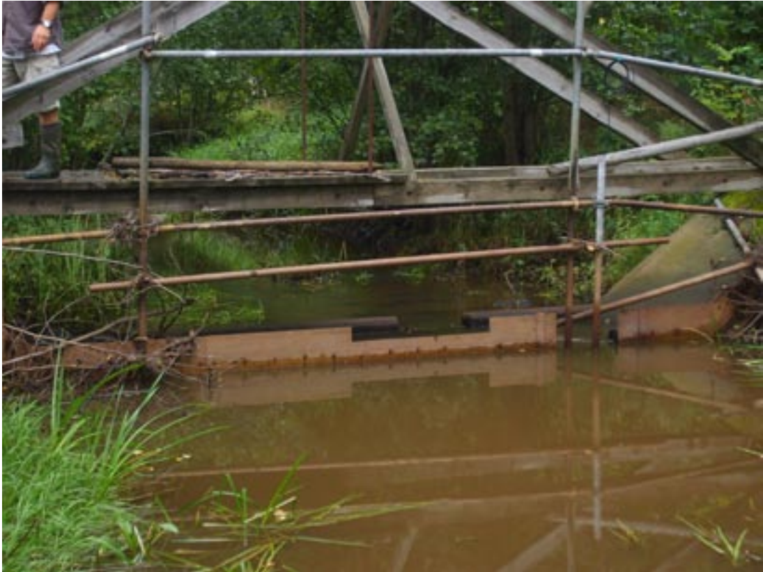
Figure 2-46. Close-up view of the submerged notch at PSM000364.
