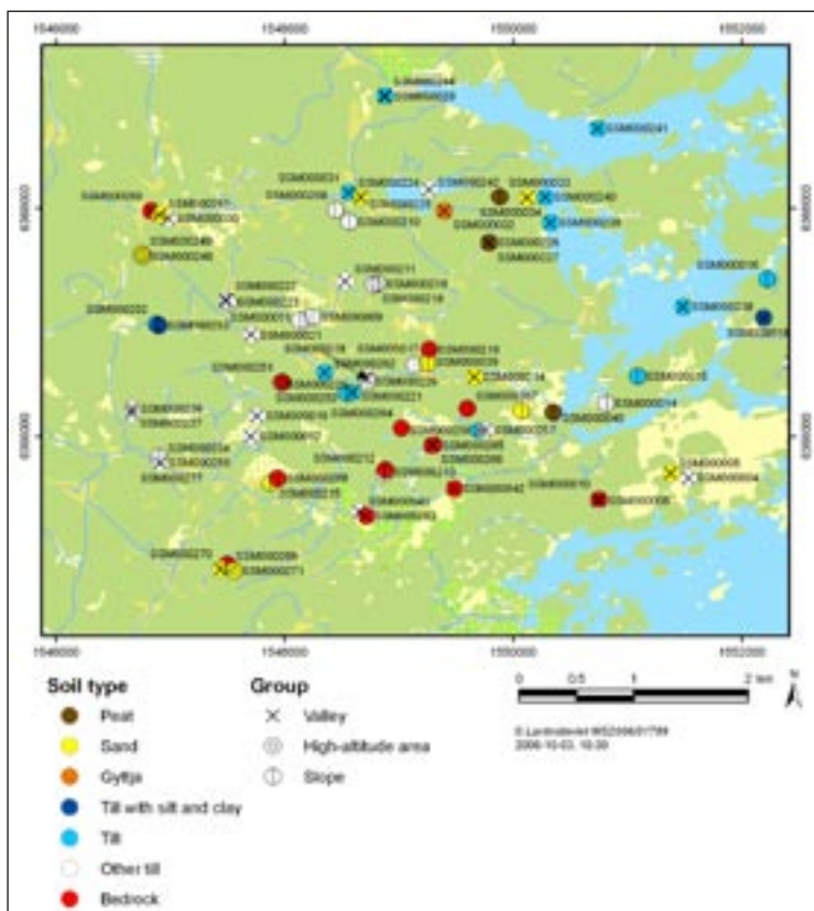
Figure 3-31a. Overview map (top) and a map of groundwater monitoring wells, classified according to topography and type of QD at well-screen depth.
