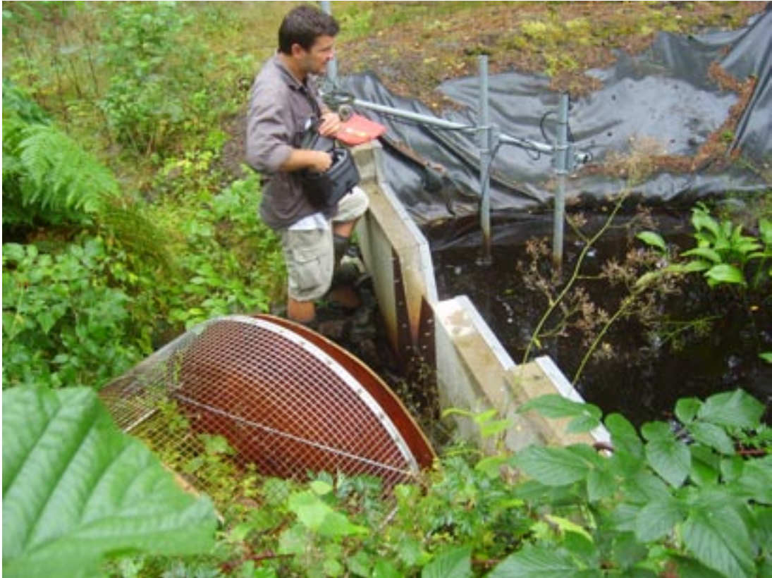
Figure 2-39. V-notch weir at gauging station PSM000341. The net has been removed to allow control measurements.
