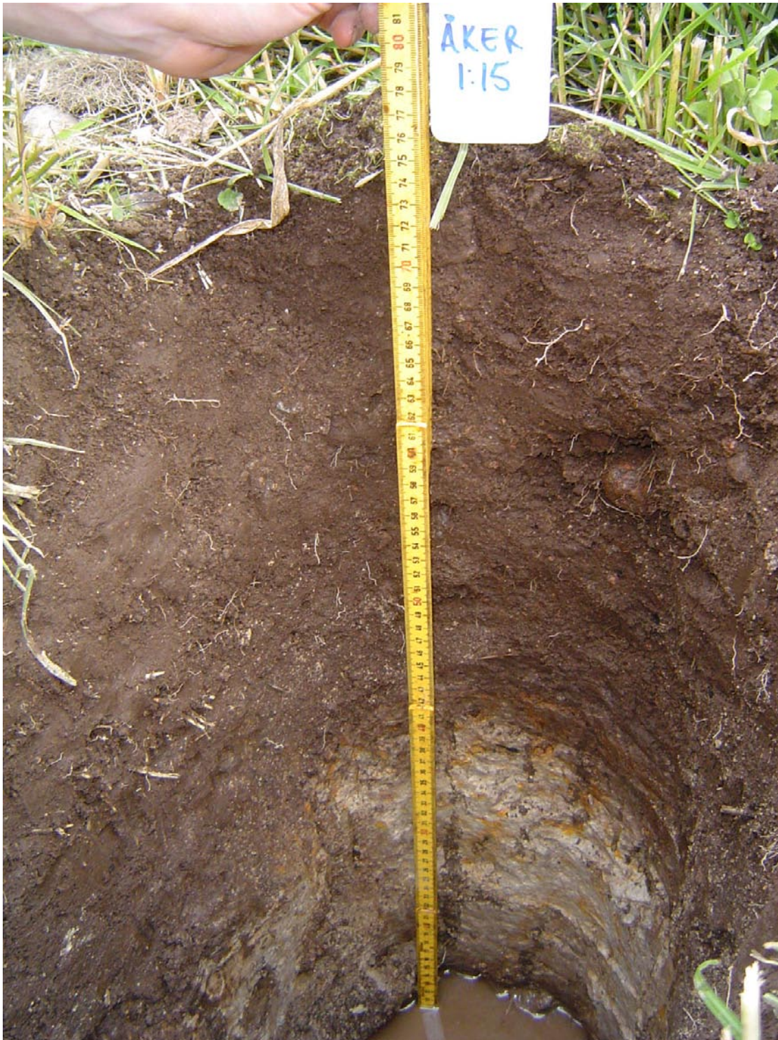
Figure 6-13. A soil profile from a Gleysol formed on clay gytja in an area used as arable land. The uppermost c 30 of the profile has a darker colour and is rich in organic matter. That layer has been affected by ploughing. The underlying layer has a greenish-grey colour with dots of rust that are typical of Gleysol.
