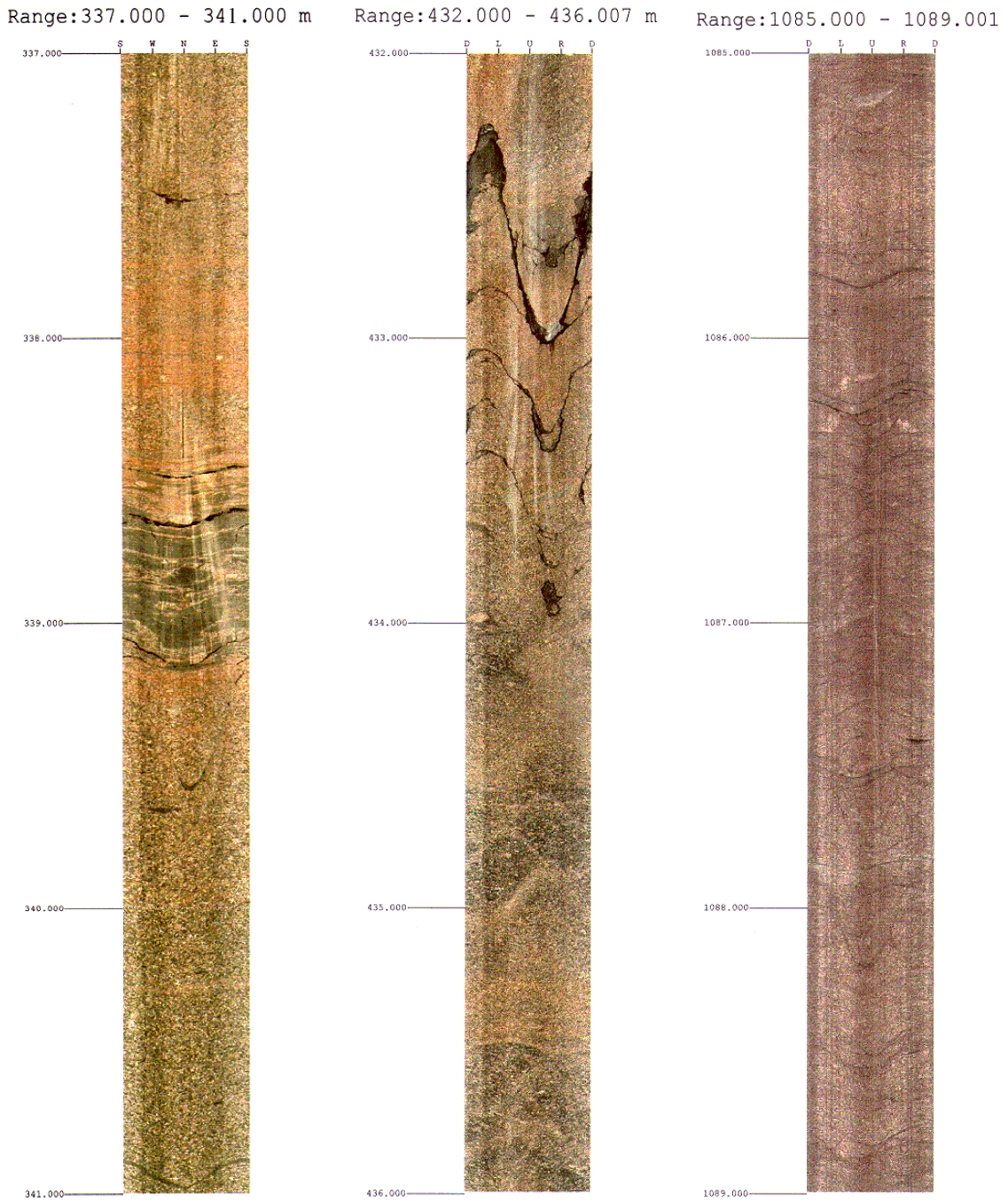
Figure 4-21. BIPS-images from those parts of borehole KLX02 where incidents with equipment jamming have occurred. After Appendix in /4-16/.
