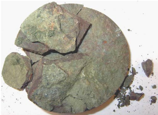
Photograph of the fracture surfaces of the drill core sample KLX04: 352.69–352.81 m.
