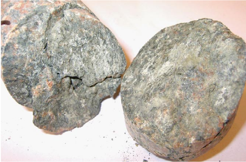
Photograph of the fracture surfaces of drill core sample KLX03: 326.94–327.04 m.
