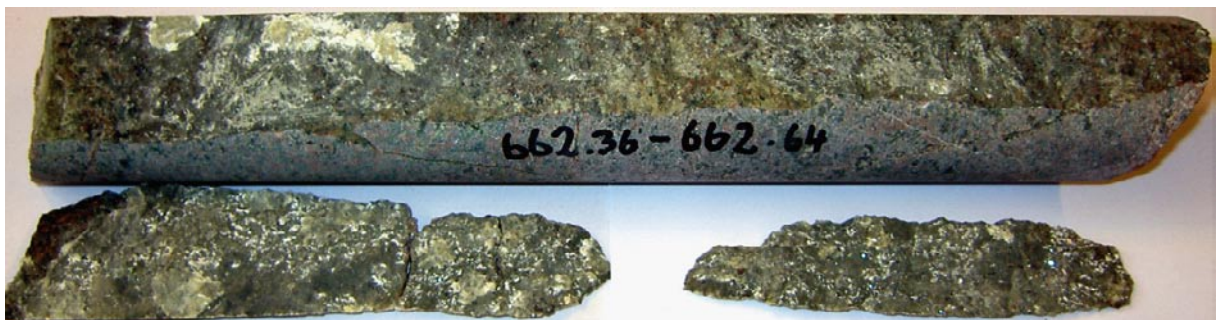
Photograph of the fracture surfaces of drill core sample KLX03: 662.33–662.65 m.
