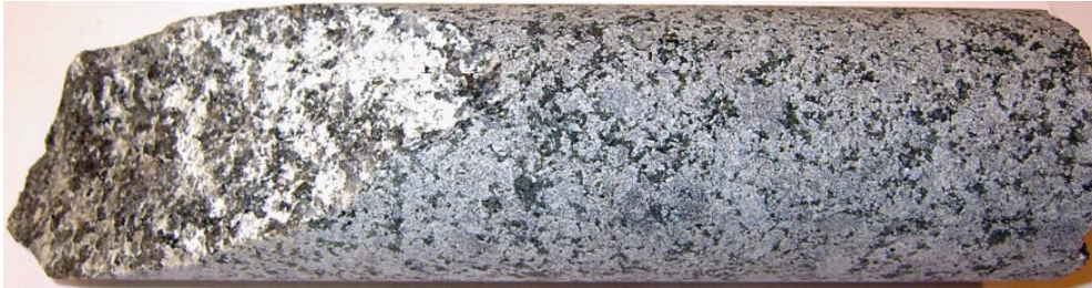
Photograph of drill core sample KLX03: 534.25–534.40 m. Gypsum have been scraped off from parts of the fracture surface.
