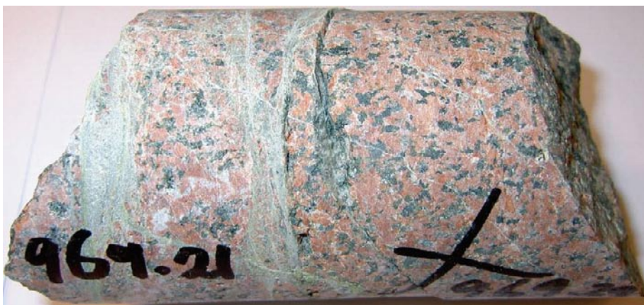
Photograph of drill core sample KLX03: 969.21–969.27 m. The fractures shown are dominantly filled with prehnite.
