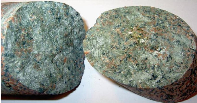
Photograph of the fracture surfaces of drill core sample KLX03: 969.21–969.27 m.
