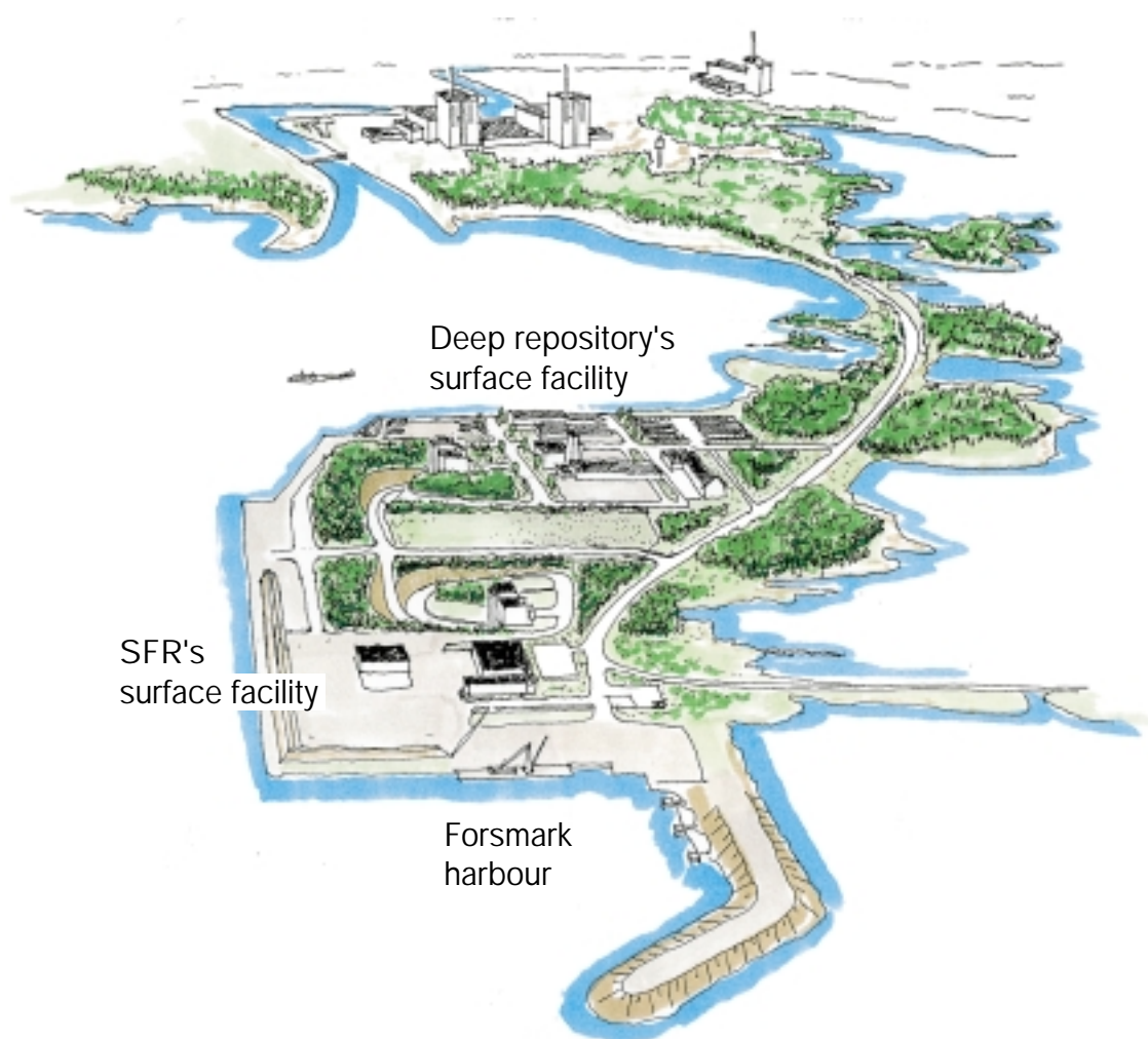
Figure 4-5. Possible layout of the deep repository's surface facility at SFR. The surface facility has been positioned between the existing buildings for SFR at the harbour and the Forsmark NPP.
