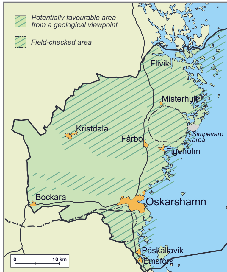
Figure 6-2. Potentially suitable areas for a deep repository in Oskarshamn Municipality. Field checks have been performed on the Simpevarp Peninsula and west of there, and in an area in the southern part of the municipality.
