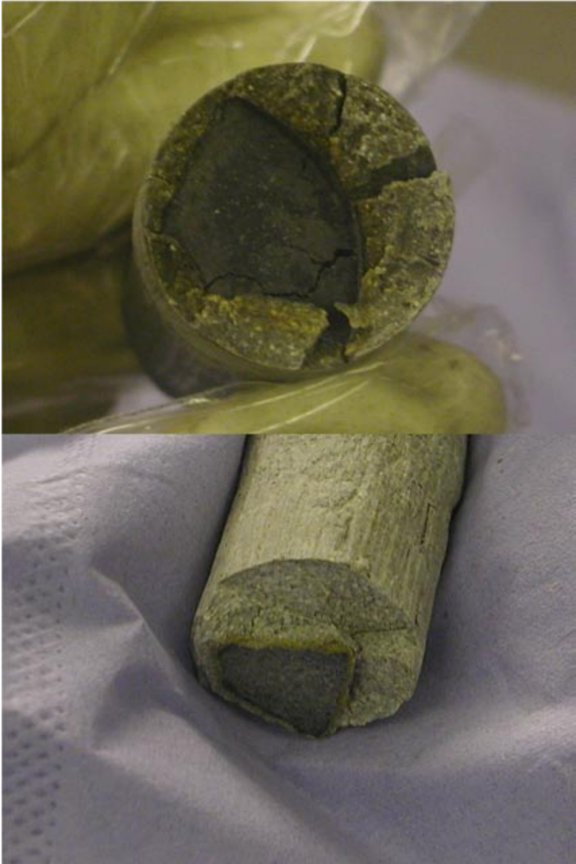
Figure A1-3. Compacted bentonite, 30°C, coupons – top: location of cast iron coupon; bottom: location of carbon steel. Samples for XRD anoxic, Raman, SEM, Mössbauer analyses were taken from the centre of the black region. For XRD oxic, FTIR, TEM, CEC and total chemical analyses samples were taken from the grey bentonite and the black zone was removed.
