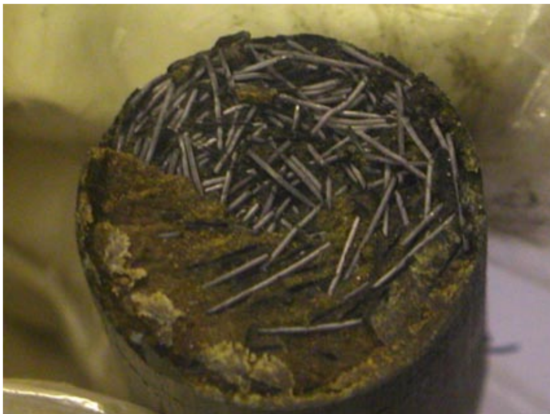
Figure A1-1. Compacted bentonite, 30°C, wires. The specimen crumbled when a slice was removed from the end of the bentonite block.
