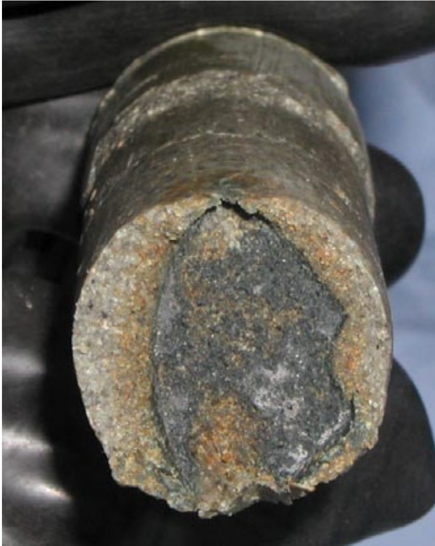
Figure A1-4. Compacted bentonite, 50°C, coupons – location of cast iron coupon. Samples for XRD anoxic, Raman, SEM, Mössbauer analyses were taken from the centre of the black region. For XRD oxic, FTIR, TEM, CEC and total chemical analyses samples were taken from the grey bentonite and the black zone was removed.
