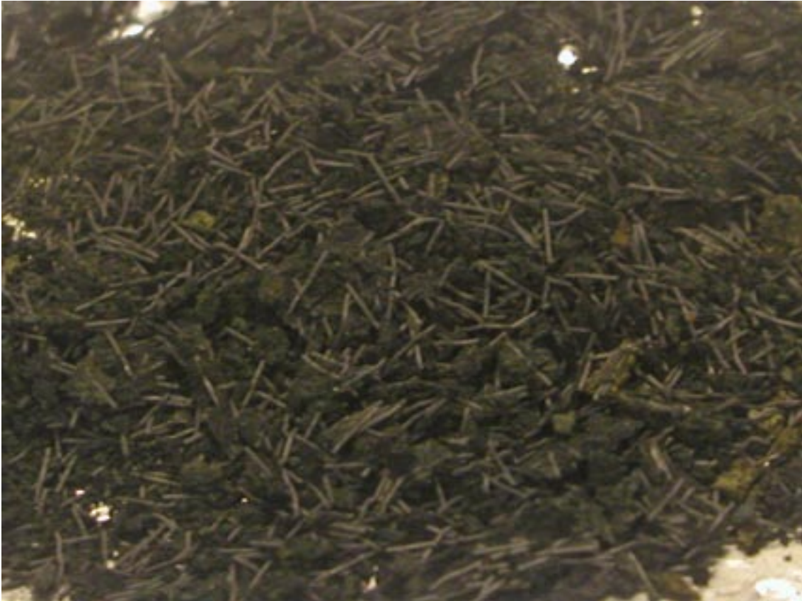
Figure A1-2. Compacted bentonite, 50°C, wires. The specimen crumbled when a slice was removed from the end of the bentonite block.
