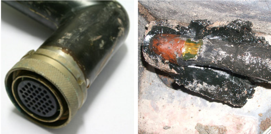
Figure 13. The polyurethane cast sealing the connection between the Gisma connector and the cable. The left image shows a new cast and the right image the state of the used.
