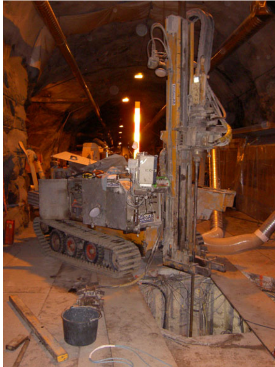
Figure 8. Rig for performing the buffer core drilling. The machine is designed for geotechnical soil sampling.
