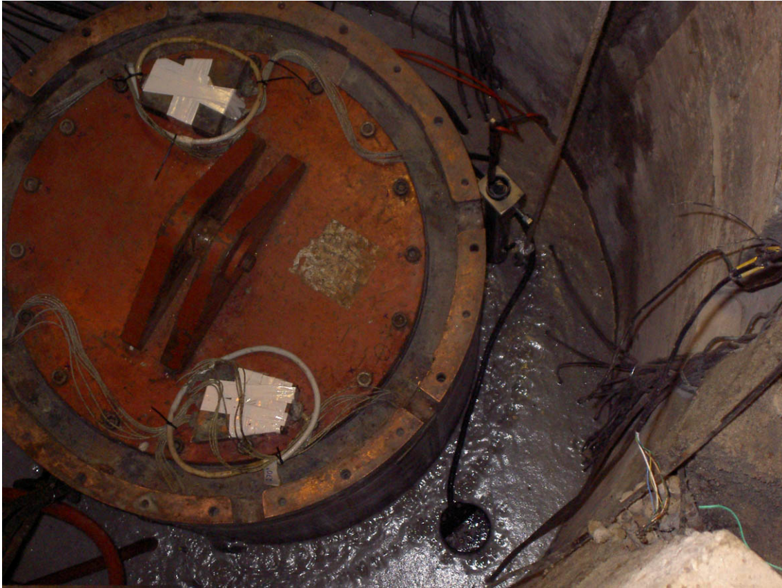
Figure 22. The buffer disintegration system in operation. The canister is visible in the center.
