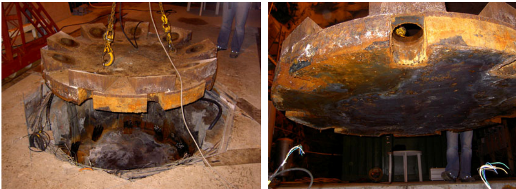
Figure 5. The steel lid is lifted from the deposit hole. Some corrosion is visible on the side and underneath the lid.
