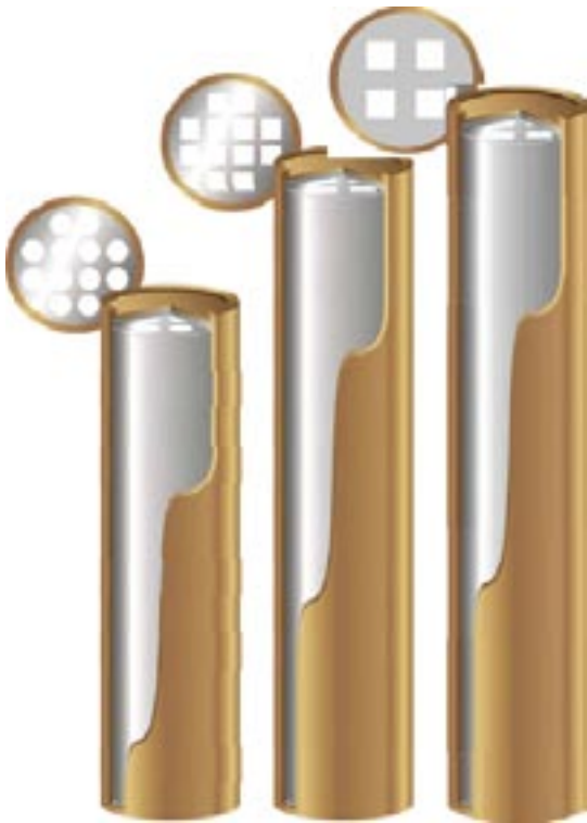
Figure 3-1. Copper-iron canisters for the spent fuel from the Loviisa 1-2 (VVER-440), Olkiluoto 1-2 (BWR) and Olkiluoto 3(EPR) reactors (from left to right; figure taken from /Raiko 2005/).
