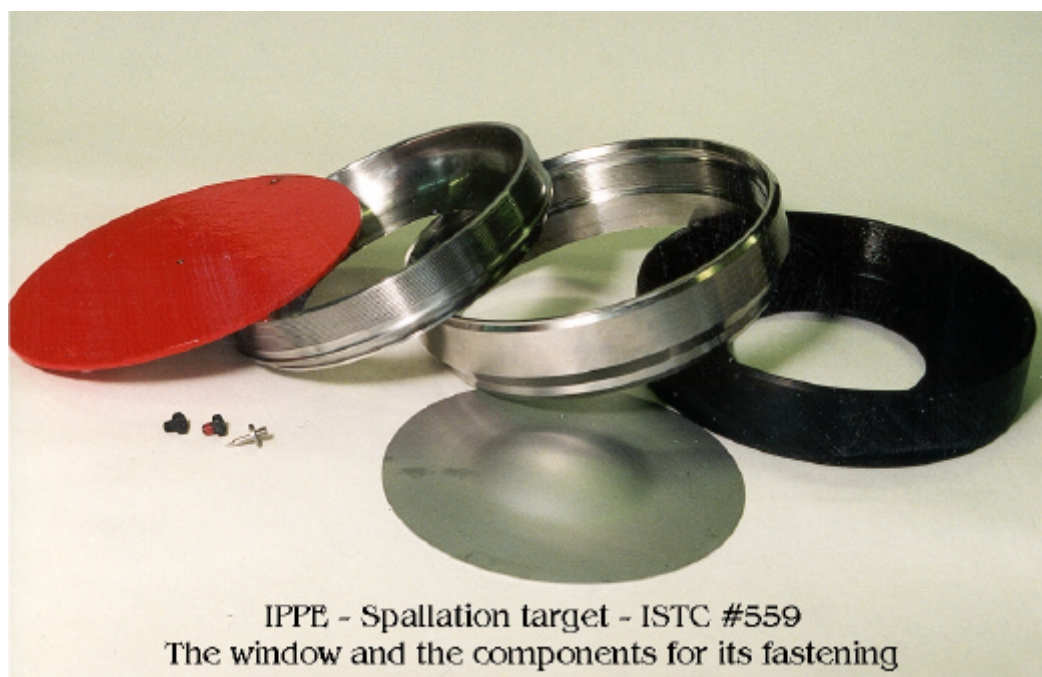
Figure 8-3. The spallation target window with some constructional components.
