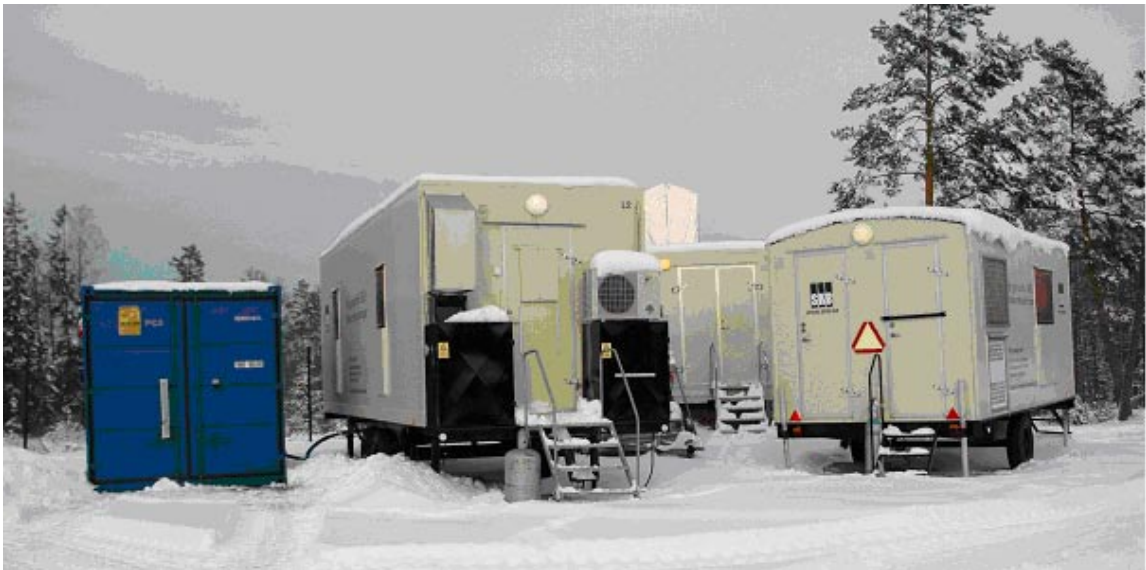
Figure 4-1. The mobile units used at KLX13A; from left container for collecting the water from the borehole, laboratory unit, hose unit with downhole equipment and a unit for computer work.
