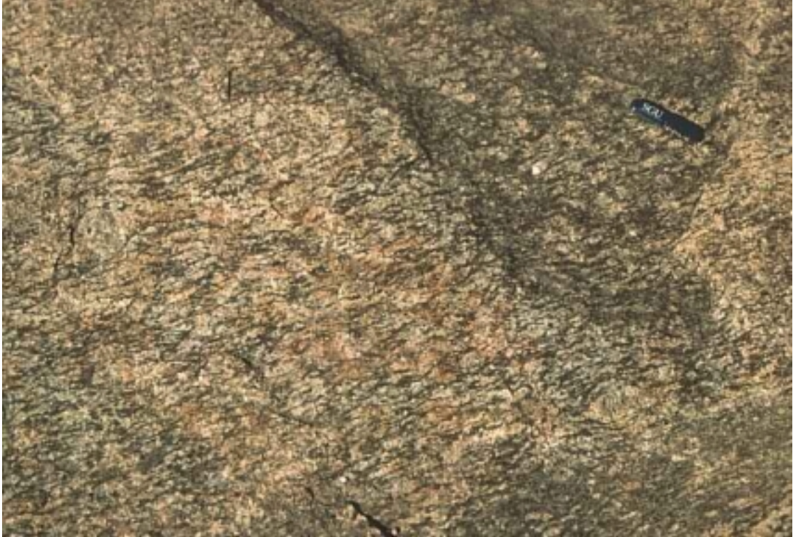
Figure A1-6 Outcrop with porphyric granodiorite in the cave area, observation no. BOD980013.
