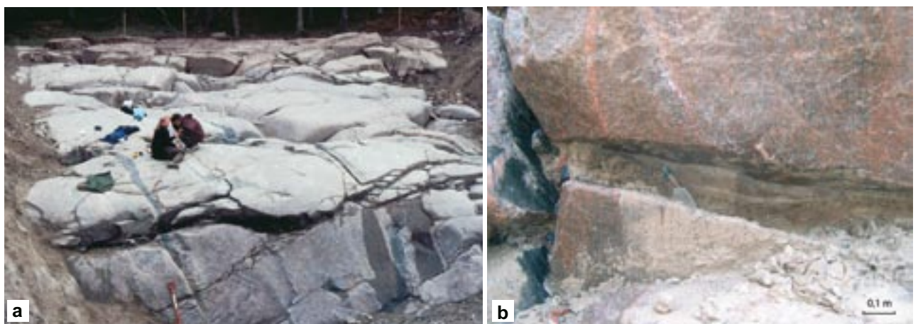
Figure 4-6. Character of bedrock and fractures at drill site 5, Forsmark. The site was originally covered with till that has been removed. (a) Glacially smoothed and striated bedrock. Freshly fractured bedrock is common along the exposed surface. The major fracture in the foreground, which lacks signs of glacial abrasion, was filled with laminated silty sandy sediment. (b) Laminated silt in an open fracture in the north-western part of the excavated area at drill site 5.
