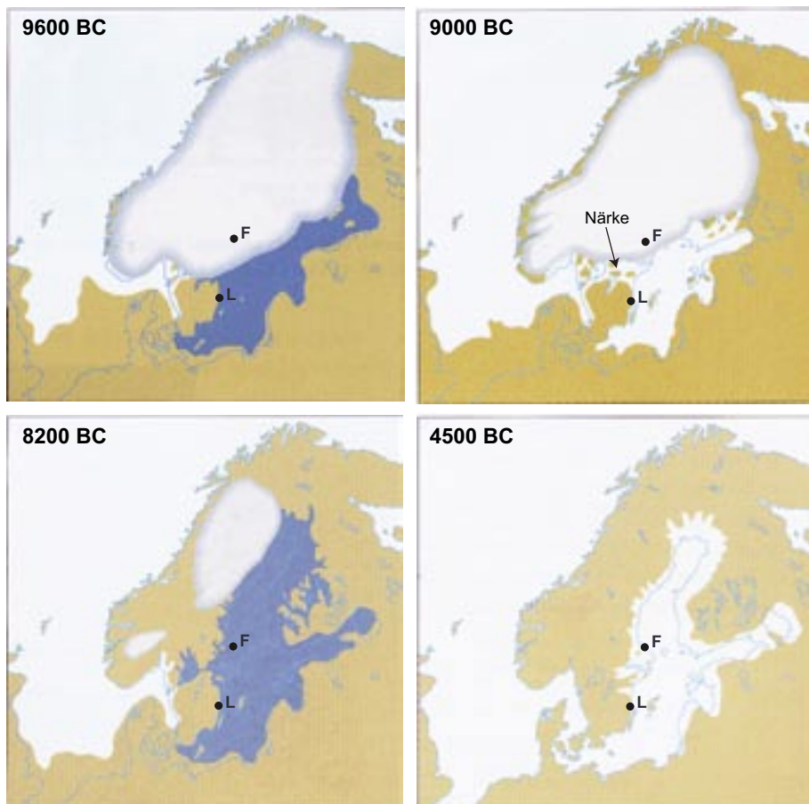
Figure 3-11. Four main stages characterise the development of the Baltic Sea since the latest deglaciation: A) the Baltic Ice Lake (13,000–9500 BC), B) the Yoldia Sea (9500–8800 BC), C) the Ancylus Lake (8800–7500 BC) and D) the Littorina Sea (7500 BC-present) (modified from /Fredén 2002/). “F” and “L” shows the location of Forsmark and Laxemar-Simpevarp, respectively. Fresh water is symbolised by dark blue and marine/brackish water by light blue.
