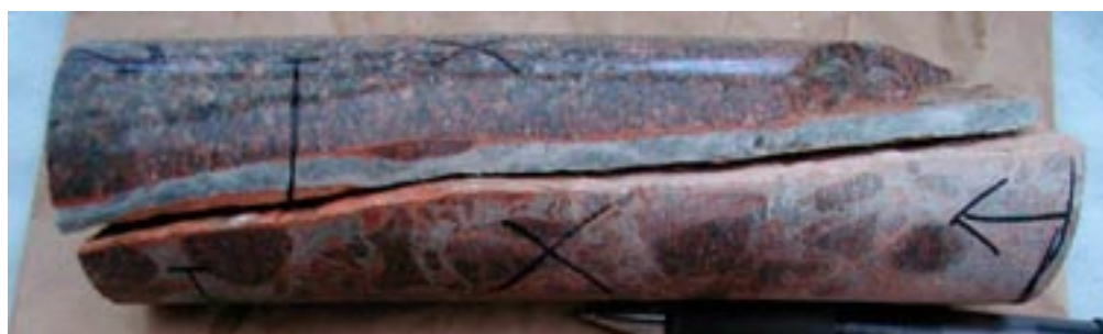
Figure 2-21. Laumontite- and calcite-sealed fault breccia in KFM04A (347.32–347.50 m) at Forsmark, within which a rock fragment has been dated using the ^{40}\text{Ar}/^{39}\text{Ar} K-feldspar technique.
