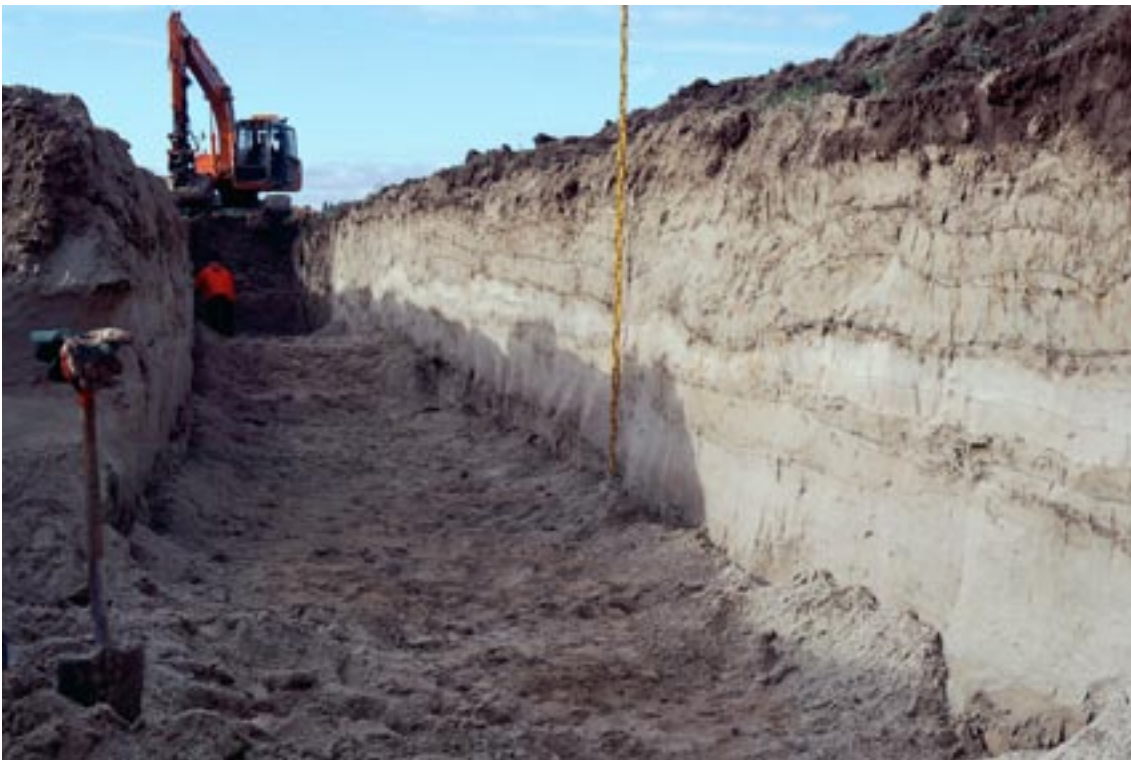
Figure 4-5. Section along a trench that is typical of the stratigraphy along the Börstil esker to the south-east of Forsmark. The section shows a bed of fine sand and coarse silt covered by a bed of clay-laminated silt. Extended excavation revealed loosely packed and saturated glaciofluvial sand to a depth of at least 5 m. Although the stratigraphy is considered to have been highly susceptible to liquefaction, if it had been saturated with water, no disturbances related to seismically induced liquefaction were discovered here or elsewhere along the esker.
