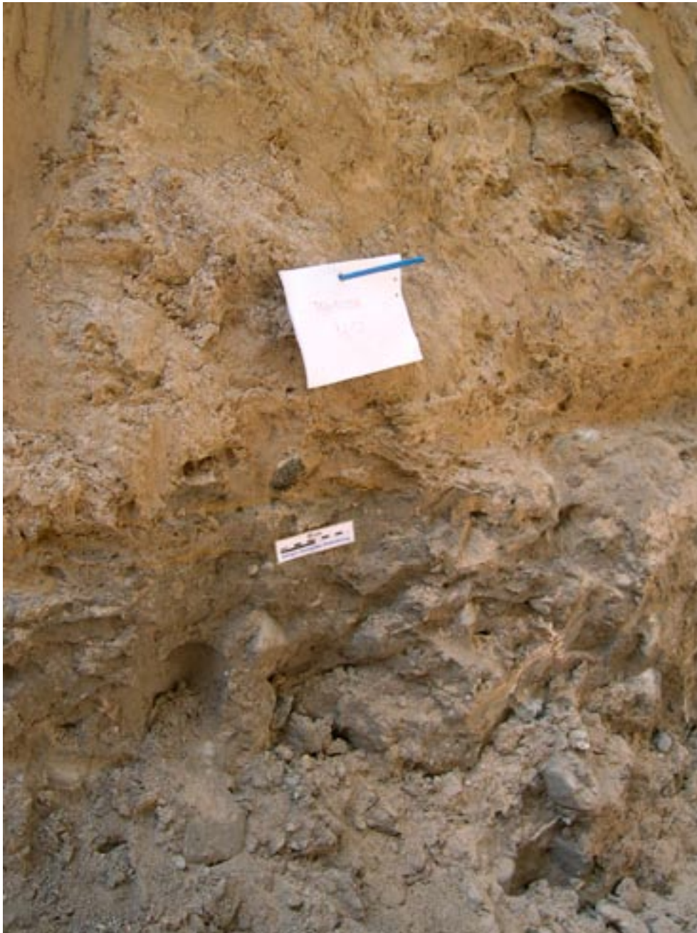
Figure 3-13. Due to erosive contact between the two till-beds, sharp-edged lumps of clayey till intercalate into the base of overlying sandy-silty till (PFM002581).
