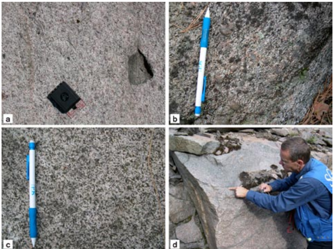
Figure 2-25. Character of well-preserved rock types in the Laxemar-simpevarp area. a) Ävrö granite with a granodioritic composition. Note the intermediate to mafic enclave in the right part of the picture. b) Characteristic appearance of equigranular quartz monzodiorite. c) Ävrö quartz monzodiorite. Note the darker colour due to higher content of dark minerals compared with the granodioritic variety in (a). d) Diffuse transition between finely porphyritic, grey Ävrö granite (upper part) and equigranular, medium-grained red granite (lower part). The geologist in the photograph is pointing at the diffuse transition.
