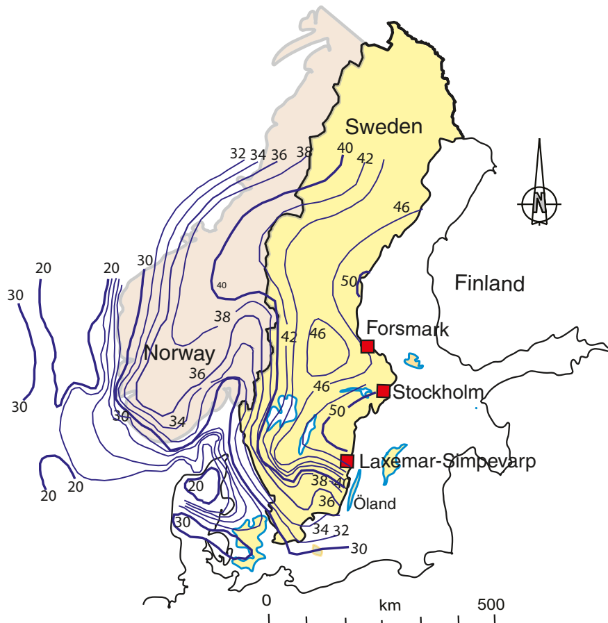
Figure 2-13. Crustal thickness contours in Sweden and Norway based on the compilation in /Kinck et al. 1993/. These contours are in two-kilometre intervals.
