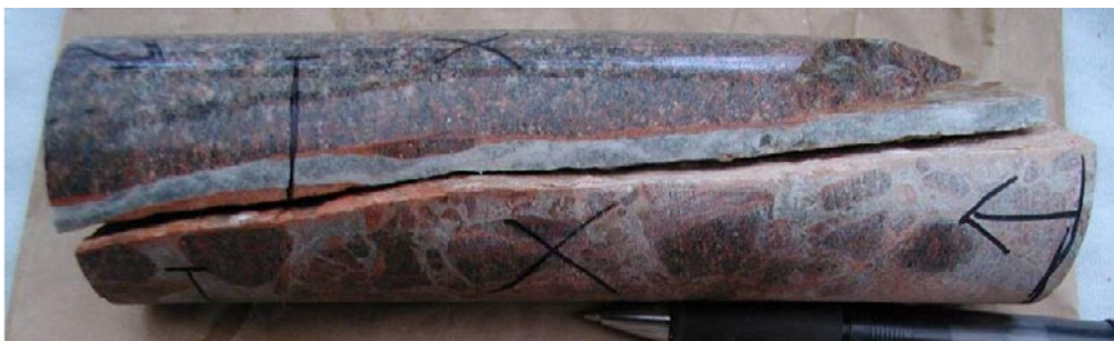
Figure 5-7. Laumontite and calcite sealed breccia from KFM05A 347.32–347.50 m. The diameter of the drill core is c 5 cm.
