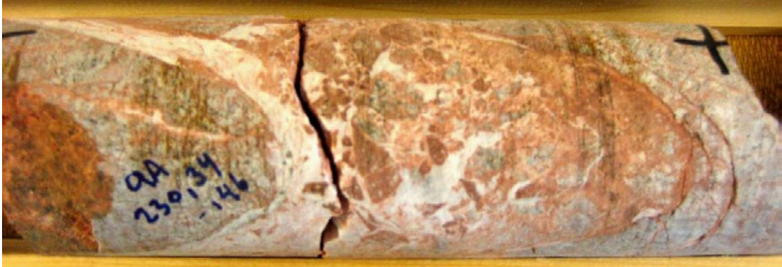
Figure 5-11. KFM09A 230.34–230.46 m; calcite and laumontite sealed breccia. The diameter of the drill core is c 5 cm.
