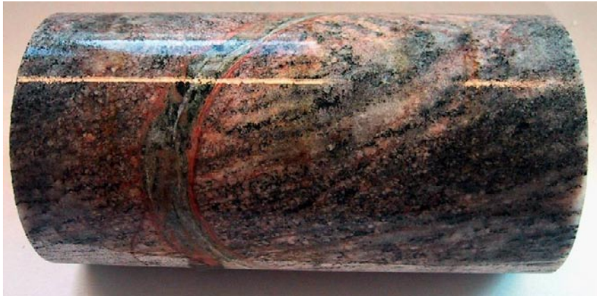
Figure 5-9. KFM08A 187.77–183.88 m; fracture sealed with adularia, quartz, prehnite, calcite, fluorite and albite. The diameter of the drill core is c 5 cm.
