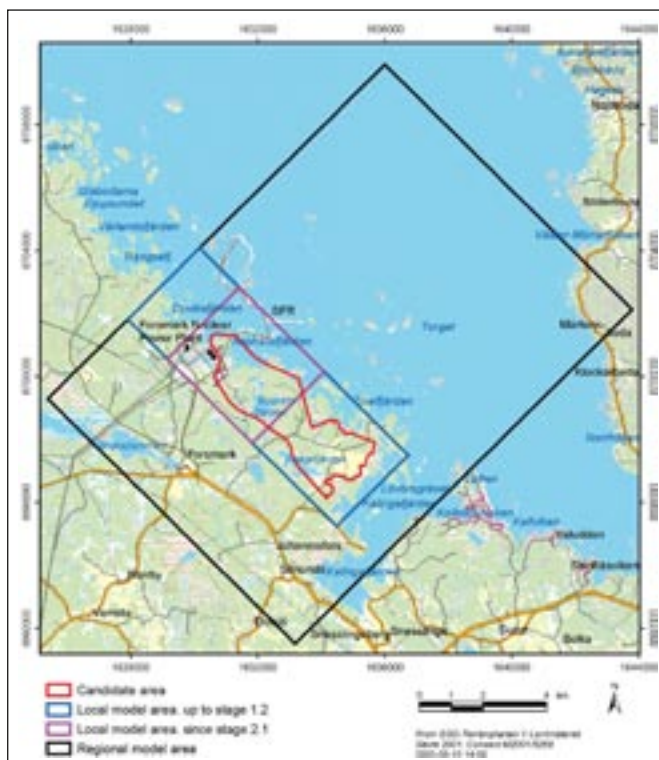
Figure 3-2. Regional (black) and local (purple) model area in stage 2.2. The regional model area is the same as in versions 0, 1.1 and 1.2 and 2.1. The local model area is smaller than in version 1.2 (blue line) and covers the north-western part of the candidate area selected as target area for a potential repository /SKB 2005b/. Reproduced from /SKB 2006a/.
