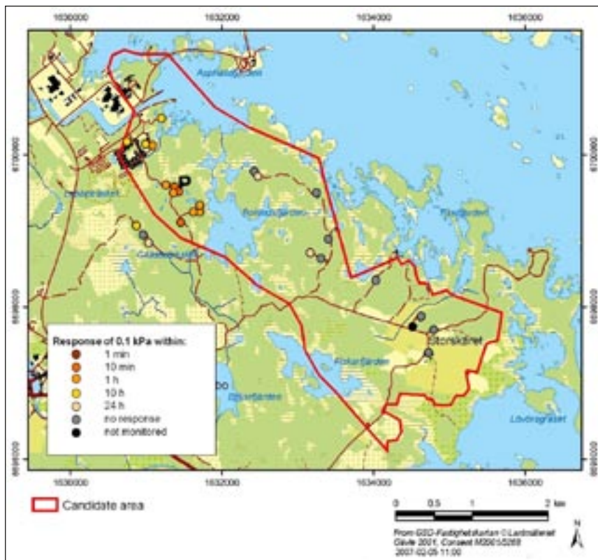
Figure 3-26. Map showing response times in the bedrock to the 2005 interference conducted in HFM01 (P). The test responses were monitored at 37 “observation points”, see /Gokall-Norman et al. 2005/.
