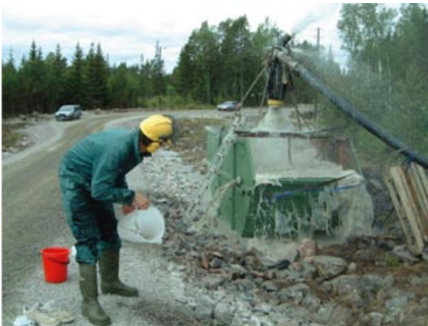
Figure 3-24. The yield in the superficial bedrock is exceptional in some boreholes. At HFM02 the yield is about 60,000 L/h. At HFM16, which is about 1 km away from HFM02, the yield is about 72,000 L/h. Reproduced from /Gentzschein et al. 2006/.
