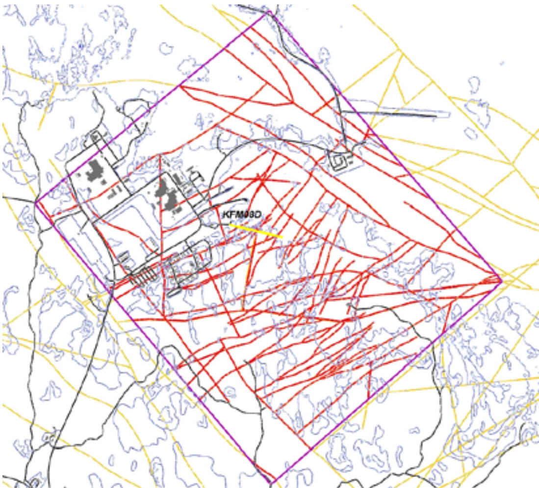
Figure D-2. Horizontal slice through the deformation zones that have been modelled deterministically in stage 2.2. The purple lines indicate the local model area in Forsmark (about 3.7 km by 3.1 km). Traces at -10 m RHB 70 are shown. Within the local area the traces of the deformation zones are coloured red, outside they are coloured orange. The location and the projected trajectory of KFM08D are indicated.
