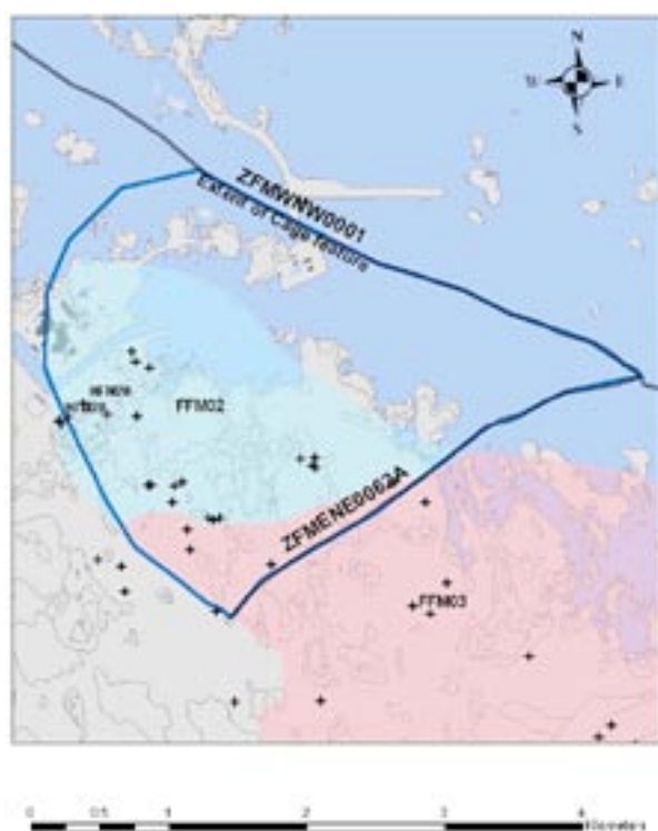
Figure I-1. The interpreted horizontal extent of the discrete features used in this study to model the “hydraulic cage phenomenon”. The crosses mark the positions of percussion- and core-drilled boreholes for which transmissivity measurements were available.
