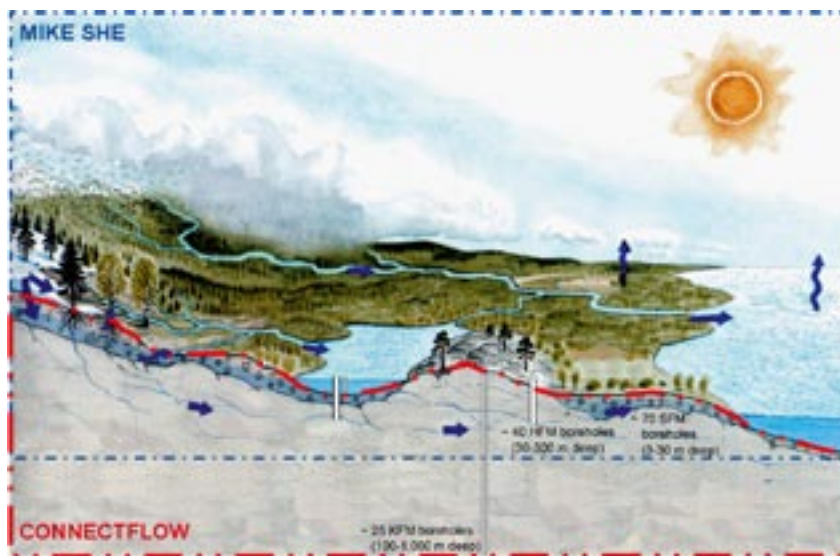
Figure 2-2. Cartoon showing how the modelling of the hydrologic cycle is divided into a surface-based system and a bedrock-based system. The former is modelled with the MIKE SHE code and the latter with the CONNECTFLOW code.
