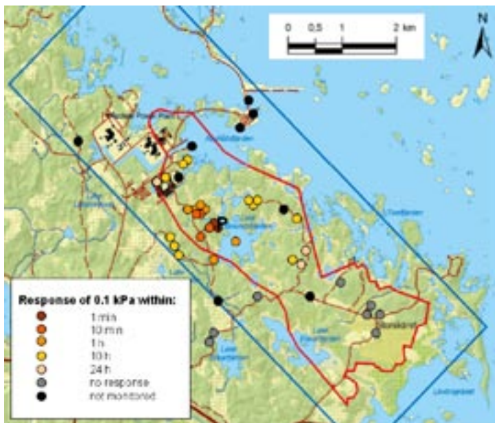
Figure 3-28. Map showing response times in the bedrock to the 2006 interference test conducted in HFM14 (P). The test responses were monitored at 71 “observation points”, see /Gokall-Norman and Ludvigson 2006/.
