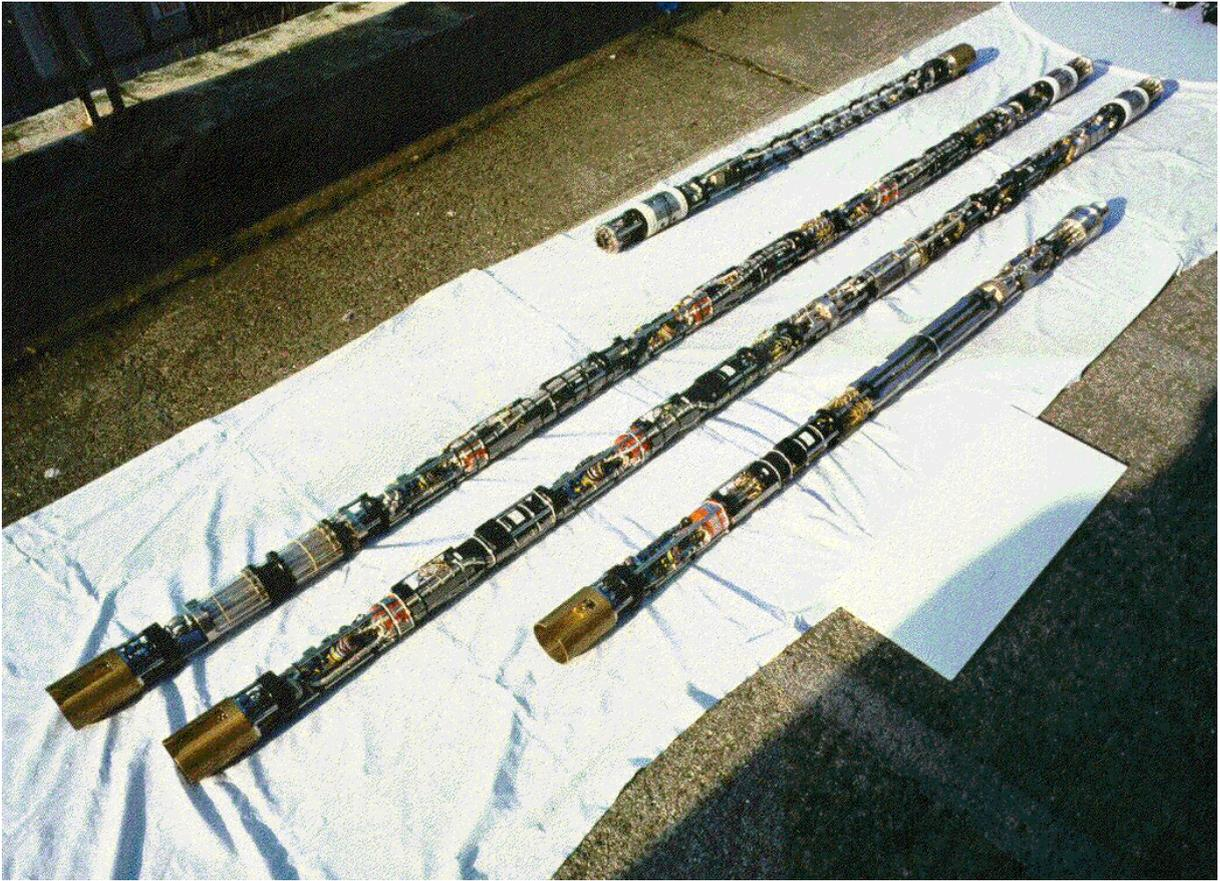
*Figure 3-3 Photograph of the CHEMLAB probe sections. The entire length of the probe is 14 metres. The different sections are coated with steel tubes which are tightly connected to each other.*
