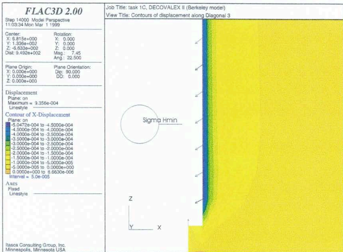
Figure 4-3 Contours of displacement on a vertical plane along the \sigma_{Hmin} axis. Arrows show the direction and the size of the displacements on the shaft wall.
