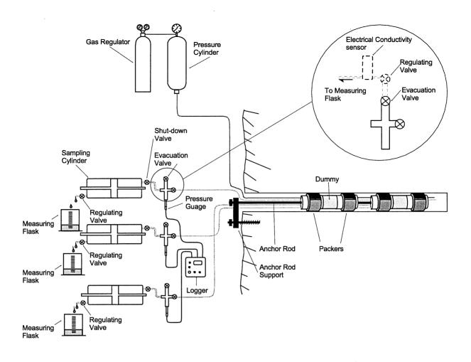
Figure A-1: Proposed experiment configuration for sampling matrix fluids. Note that the casing has not been included.
