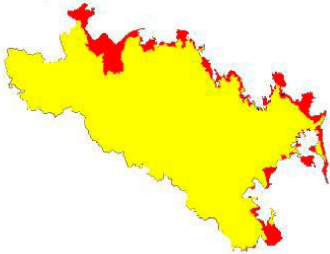
Figure 5-6. The small coastal sub-catchments with no surface water outflow into the sea (where \gamma_{\text{gw-s}} = 0 for all considered transport scenarios) are represented by the red area. Areas defined as surface water systems and the area upstream of those surface water systems are represented by the yellow area.
