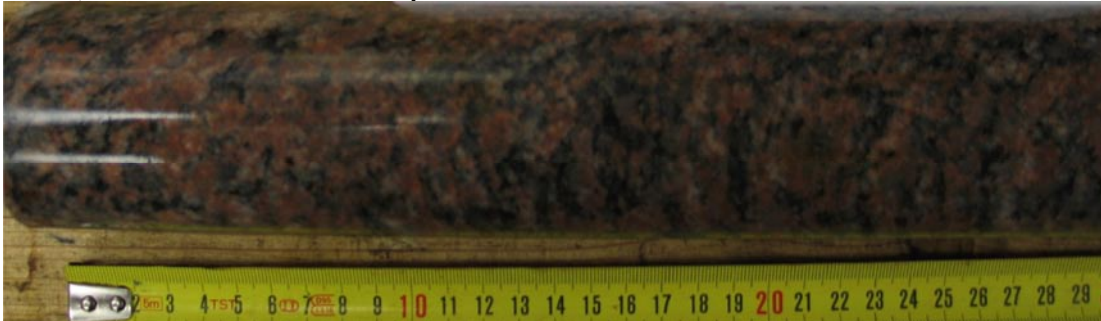
Figure G3. Photos of pilot core and overcore sample for borehole KFM02B, Level 3
