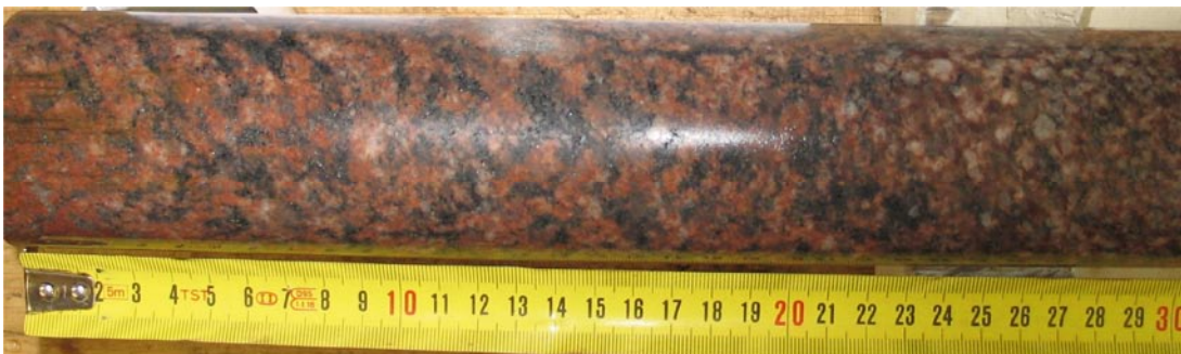
Figure G1. Photos of pilot core and overcore sample for borehole KFM02B, Level 1.
