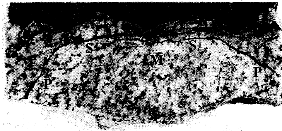
Figure 9-3 Cross-section of crack pattern caused by a triple tungsten carbide kerf cutter (Lindqvist and Rånman, 1980). S denotes side cracks, M median crack and P was named as prism crack, according to Lindqvist and Rånman.
