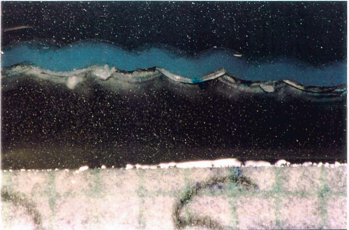
Figure 4-11. Photograph of cross section through resin impregnated replica.
