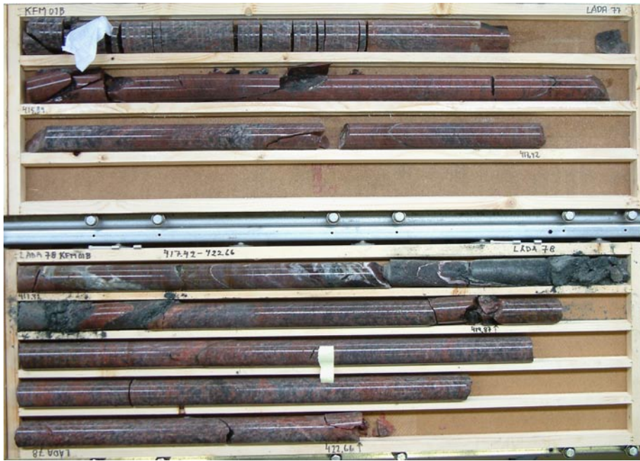
Figure 5-4. Drill core at the depth of the washout in borehole KFM01B at 419 mbl (core box no 78).
