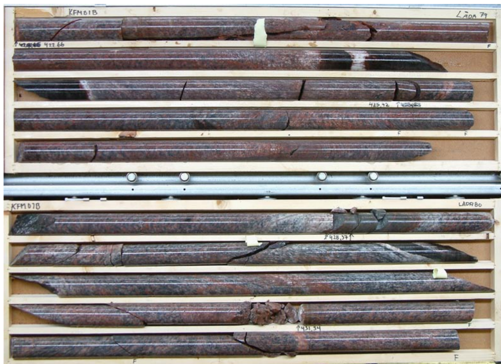
Figure 5-16. Drill core at the level of the major breakout in KFM01B at 432.0–435.2 mbl (lower core box, no 80).
