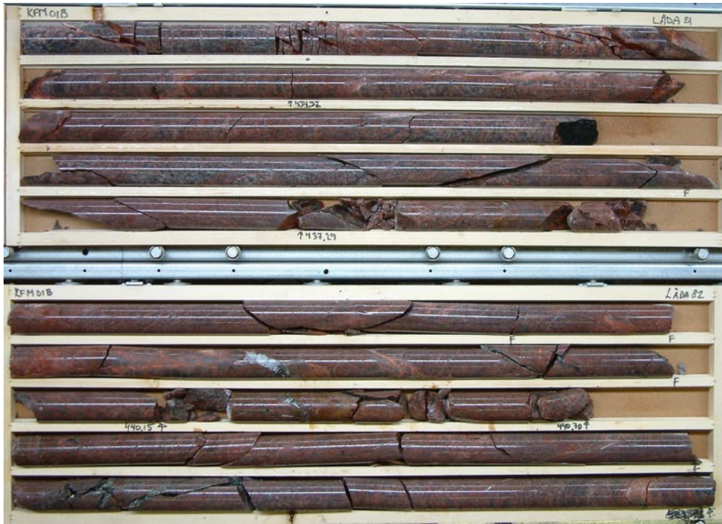
Figure 5-17. Drill core at the level of the major breakout in KFM01B at 432.0–435.2 mbl (upper core box, no 81).
