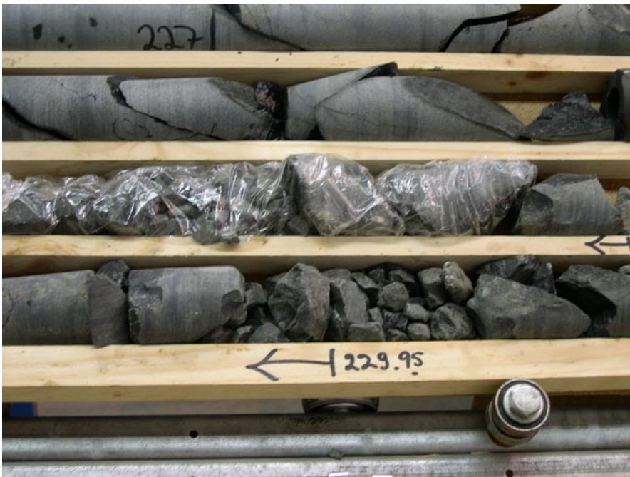
Figure 5-1. Dolerite in KLX20A. Note the strong fracturing which is characteristic along its entire length in the drill core.
