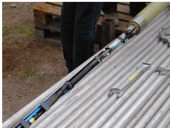
Photo 6. Packer and gauge carrier.
