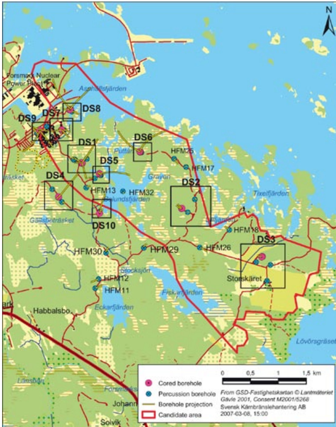
Figure 1-4. Location of drill sites and boreholes, from which data were available for model stage 2.2, at the Forsmark site /Stephens et al. 2007/.
