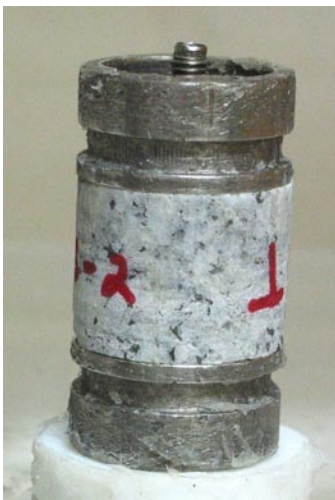
Figure 3-1. Rock core sample enclosed by end pieces to be used in a permeability measurement.
