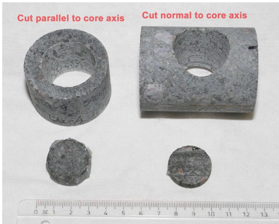
Figure 4-2. Sample core cut parallel and normal to core axis. The core slices used for permeability measurements had a 25 mm diameter.
