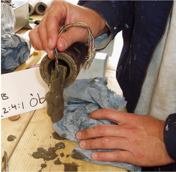
Figure 5-2. Clay and/or drill cuttings in overcored sample for test no. 2:4:1 (153.74 m borehole length).
