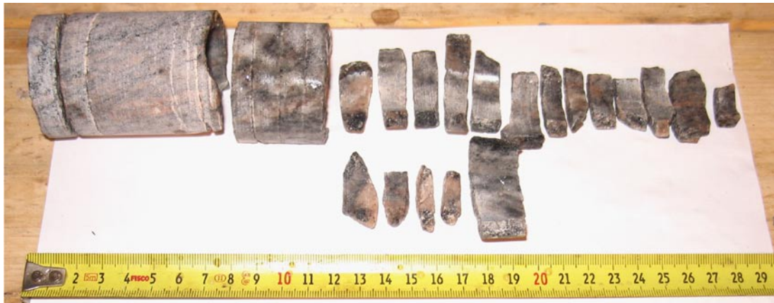
Figure 5-4. Core dinking of overcored sample for rejected pilot hole (3:3:1, 226.40 m borehole length).
