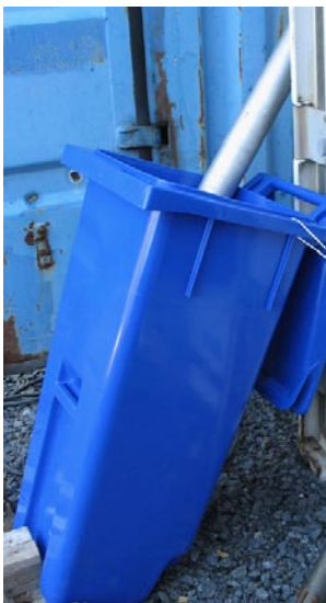
Figure 4-3. Photo of arrangement for holding the core and probe at a certain dip angle. The blue box is filled with borehole water for test Type 1 and 2 but empty for test Type 3 .
